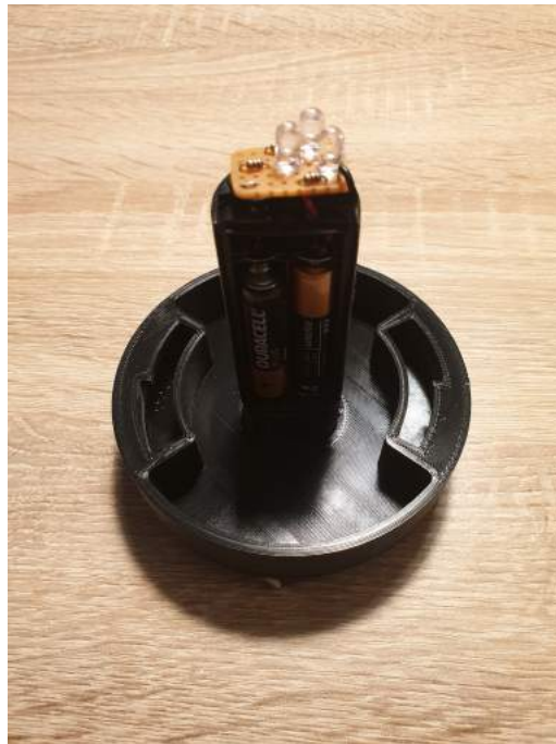
Figure 4.11: Backplate with PCB (on top) and batteries.
