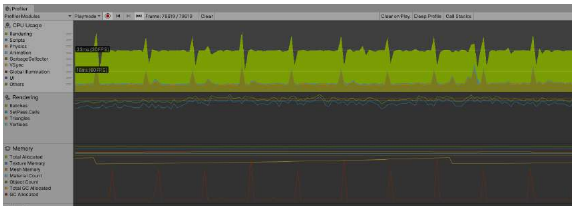
Figure 6.2: Unity profiler during VR simulation with more than 15 fires present
