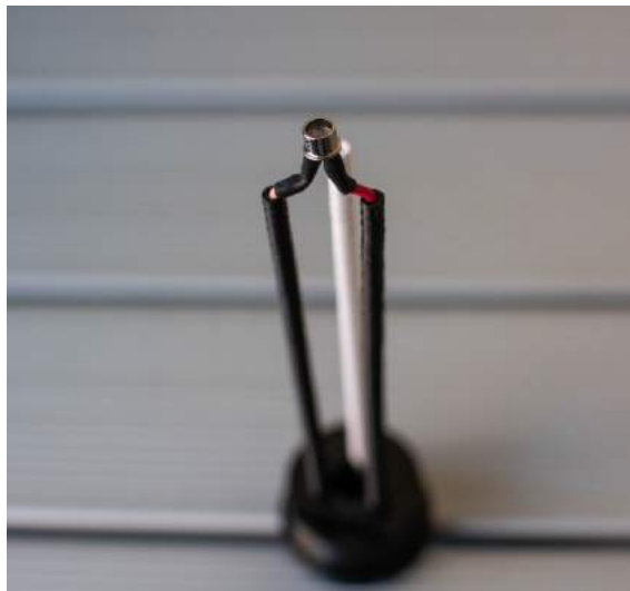
Figure 4.4: Hollow tubes attached to the base with the wires of the LDR running through them.
