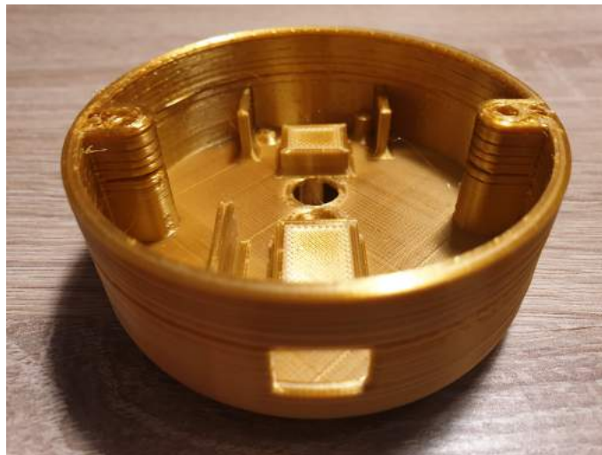
Figure 2.3: Example of under-extrusion.
