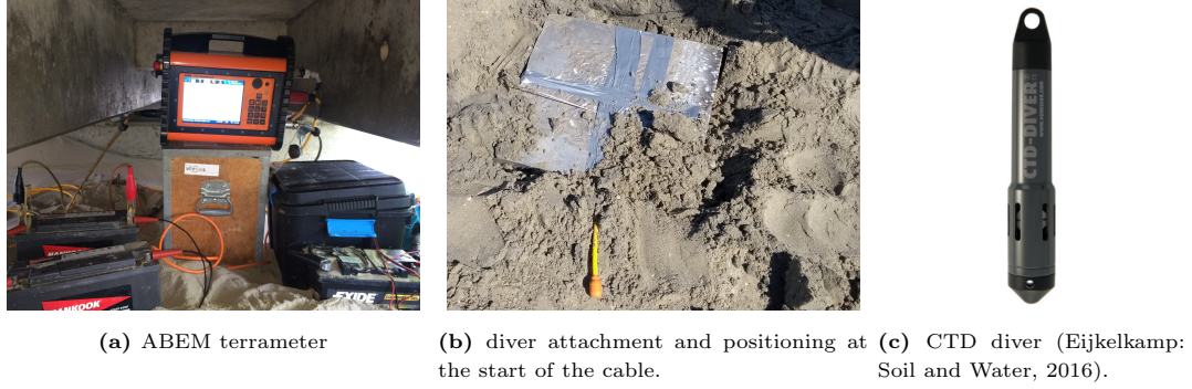
Figure 5.3: Field test set-up and equipment.
