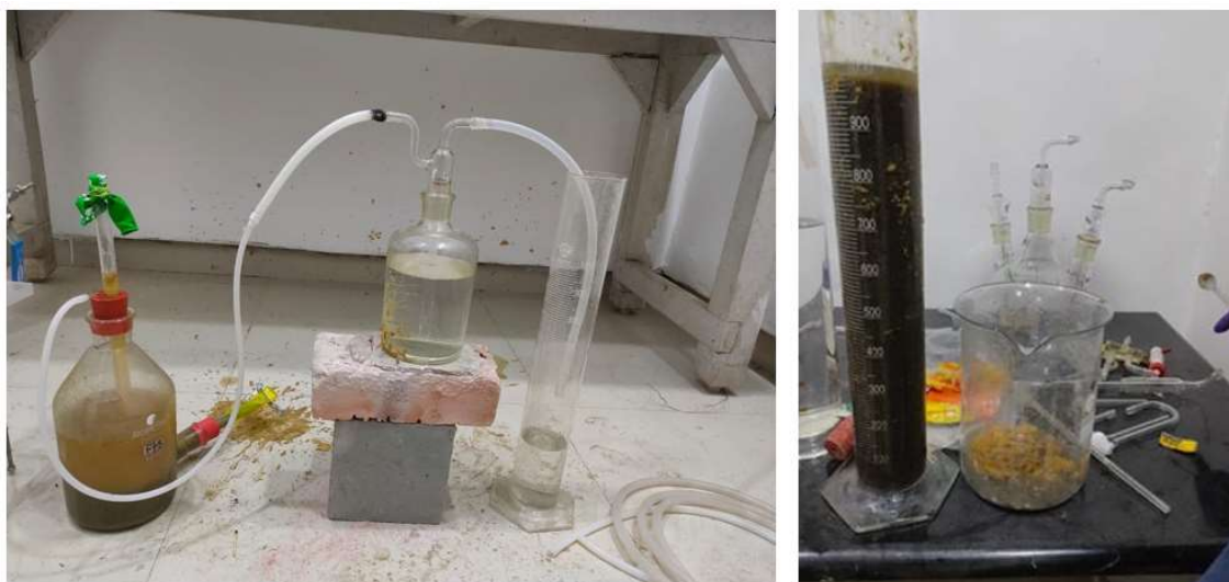
Figure 3.4 The digester set-up (left) and the different feeds (right).
