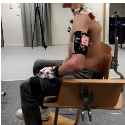
Figure 1: Placement of markers and IMU devices
