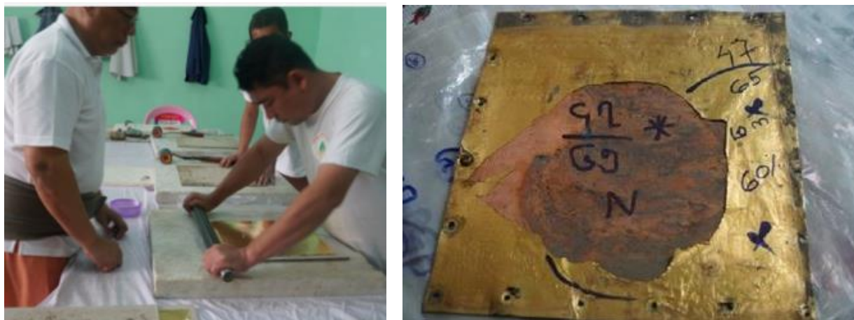
Figure 2: Left: gluing of the gold plates onto the copper next to the Shwedagon Pagoda, Right: delamination of the gold from the copper plates.
