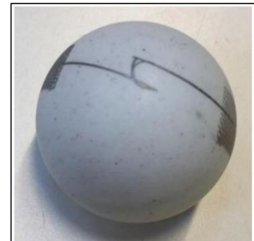
Figure 2.30: 5-axis printing on ping pong ball [75]
