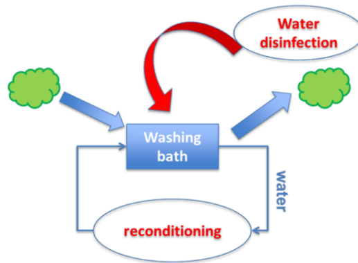
Figure 6. Schematic overview of the reconditioning treatment, i.e. off-line disinfection of process water with NaOCl (Van Haute et al. 2015).
