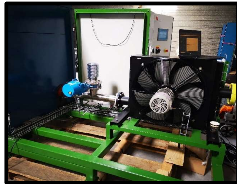
Figure 6 - Cooler & FAV on skid
