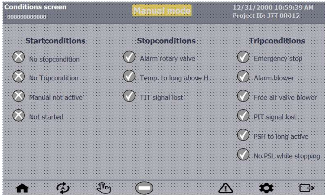
Figure 31 - HMI: Conditions screen
