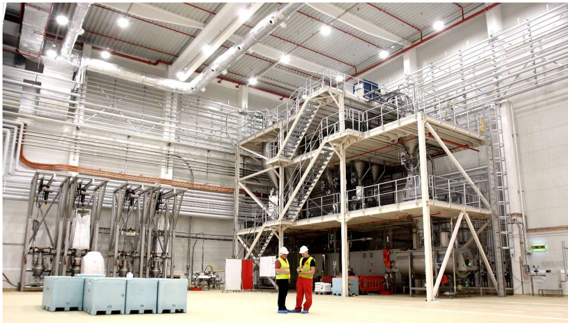
Figure 2 - General J-Tec pneumatic conveying systems
