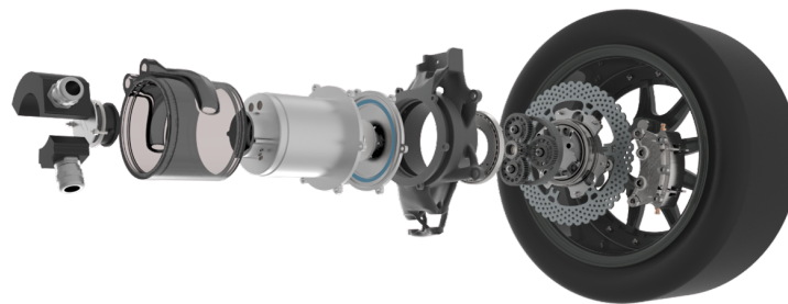
Figure 1.2: Exploded view of the inwheel of Aurora Mk II
