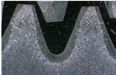
(a) Laser hardened tooth with cooling, high pressure
