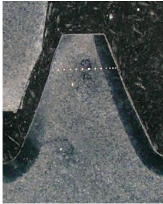
(a) Laser hardened tooth without cooling and visible tempering
