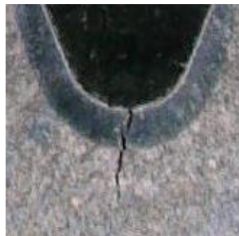
Figure 8.8: Observed crack in the tooth root for transverse velocity of 25mm/s
