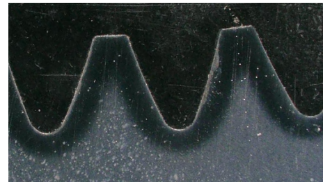
(b) Carburized teeth of the ring gear
