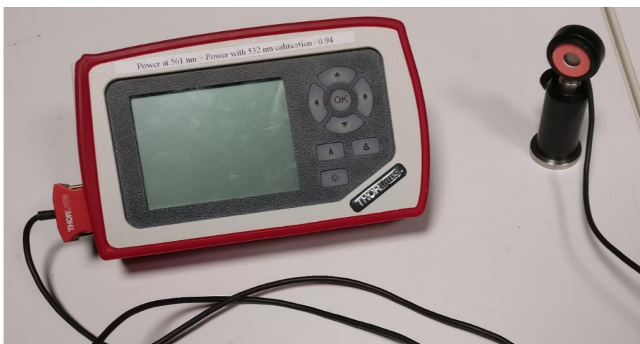
Figure 3.5: Thorlabs PM100D Power Meter & S121C Power Head
