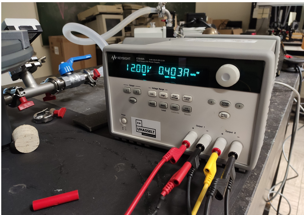
Figure 5.31: 12 V output and the corresponding current usage.
