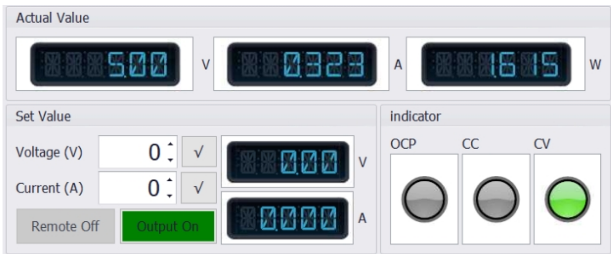
Figure 4.11: 5V power consumption on the OSCAR-QUBE.
