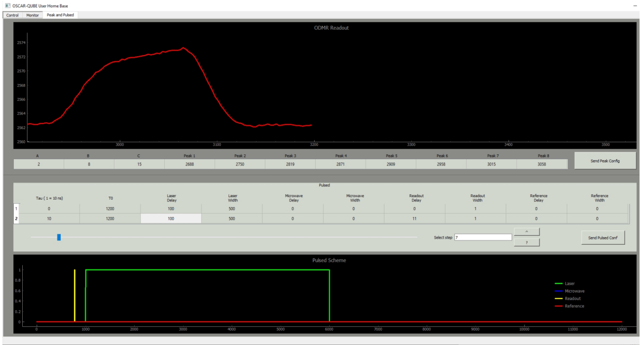
Figure 4.12: UHB showing the pulsed ODMR response.
