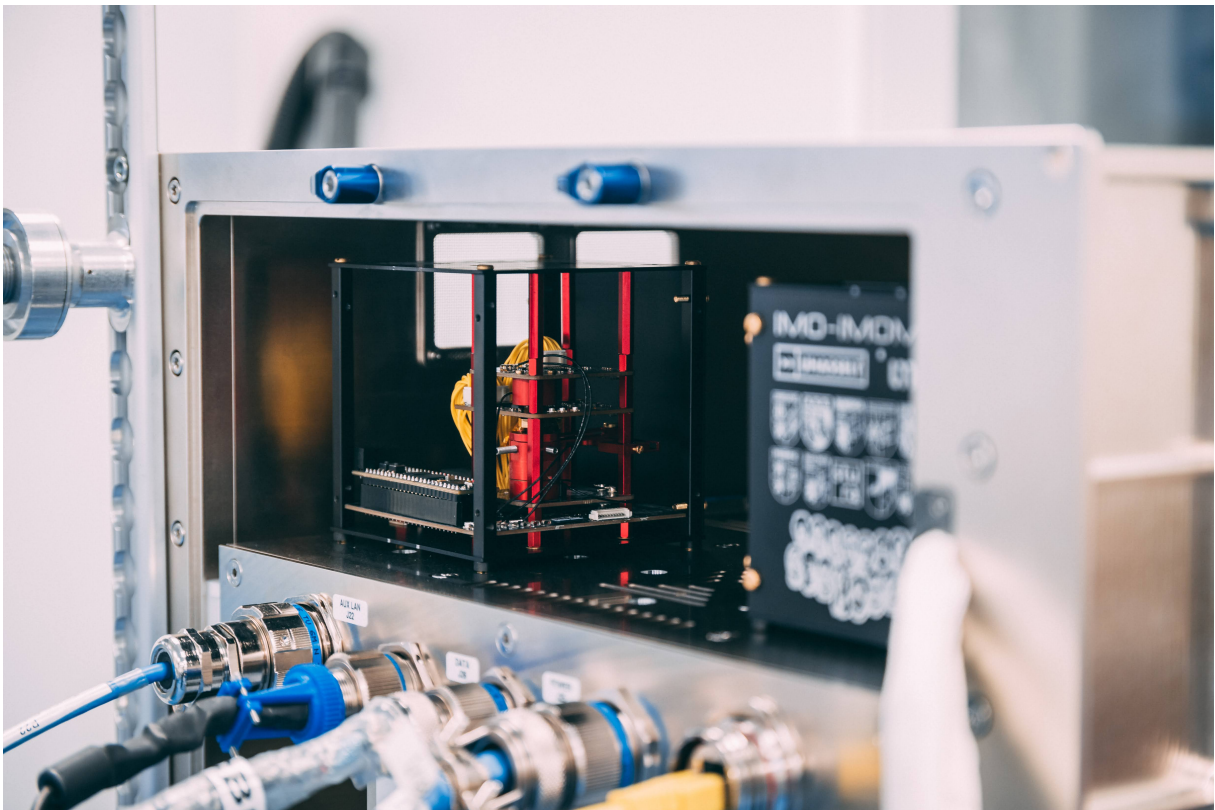
Figure D.5: OSCAR-QUBE at Space Application Services in the ICE CUBE Facility with tray closed.
