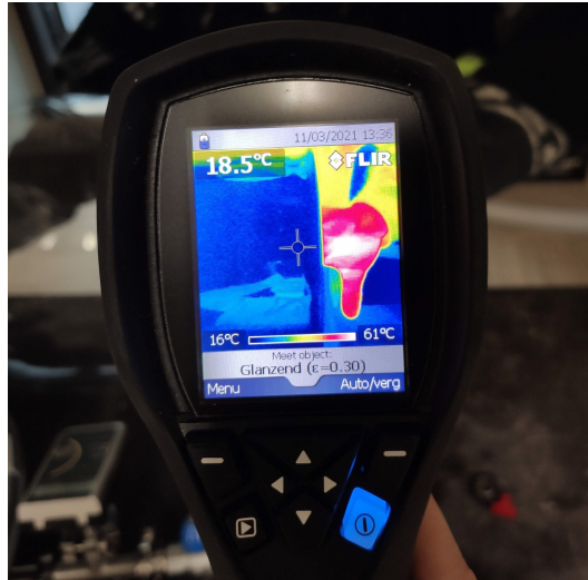
Figure 4.18: Glass acting like a mirror for infrared radiation.
