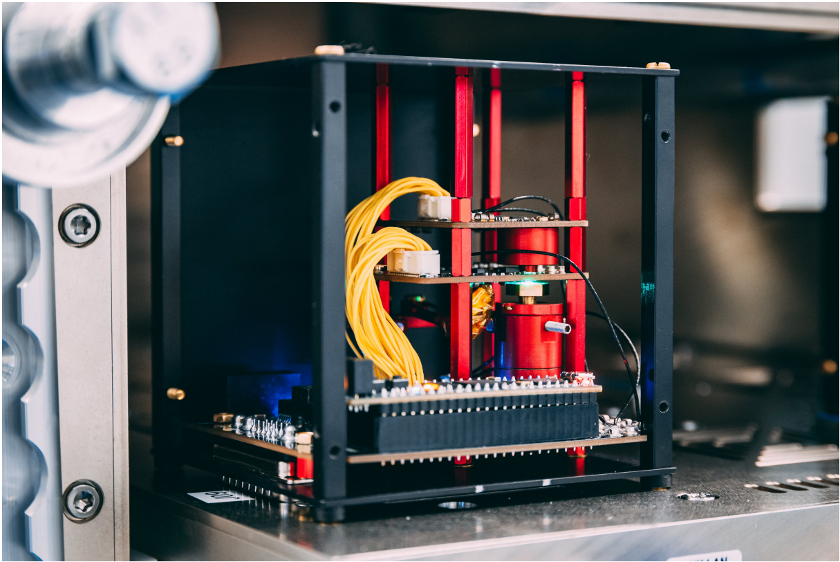
Figure D.6: Close-up of the powered OSCAR-QUBE GM at Space Application Services in the ICE CUBE Facility.
