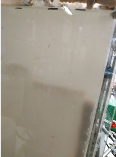
Figure B.7: Dispersed growth at the end of Phase I, after settling of the activated sludge.
