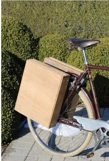
Figure 76: Angled cargo container
