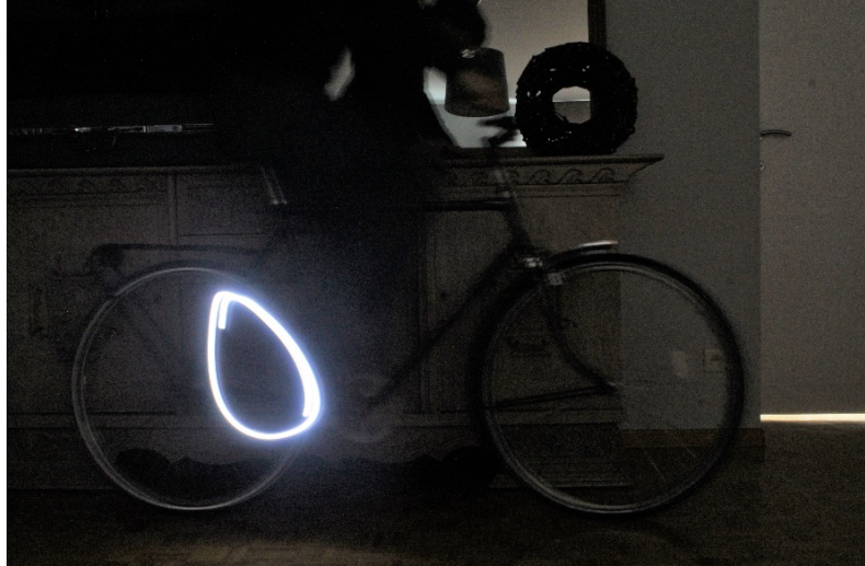
Figure 77: Long exposure photograph + LED show heel strike trajectory
