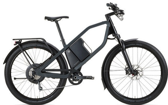
Figure 57: Frame triangle is used for battery storage (source: Klever)
