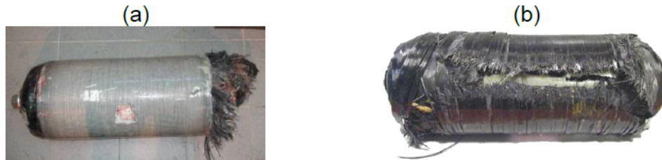
FIGURE 1.6: Vessels burst mode: dome burst (a) and cylindrical part burst (b) (13)
