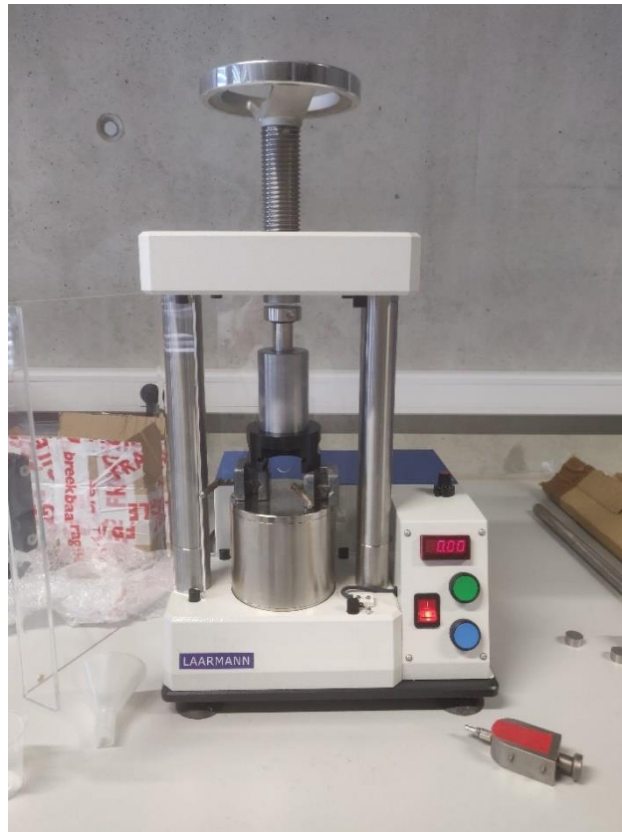
Figure 58: Pellet press for compaction of cylindrical geopolymer samples.
