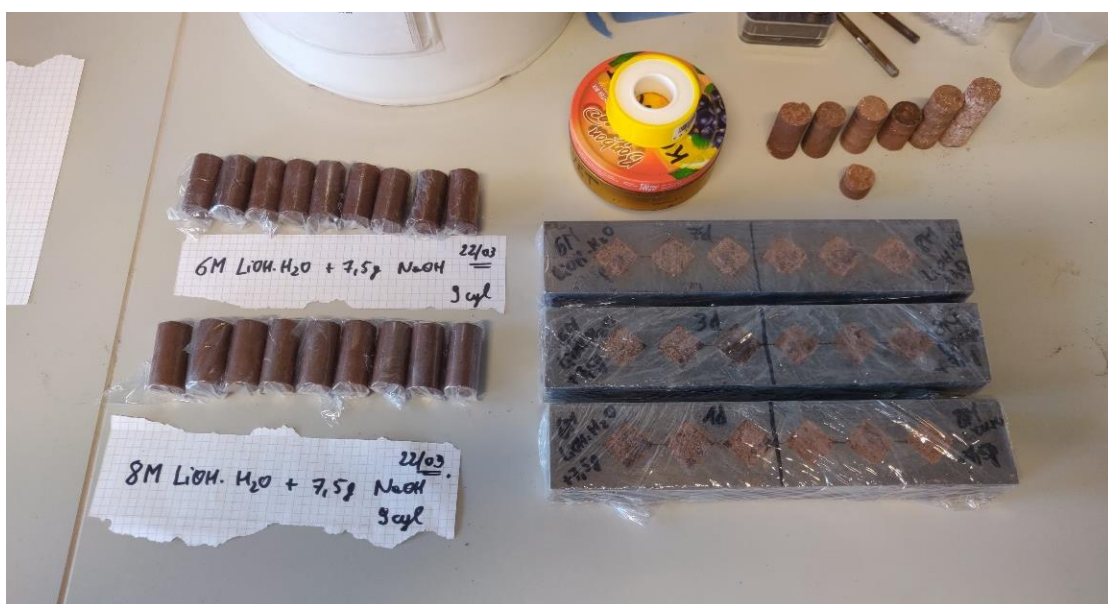
Figure 67: Prepared cylindrical and cube geopolymer samples.
