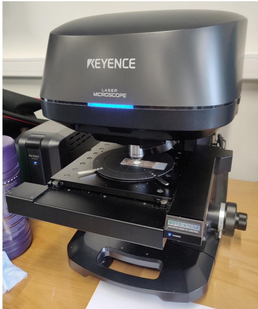
Figure 79: Keyence laser microscope for determining the effect of grinding MGS-1 and calcination of kaolinite.
