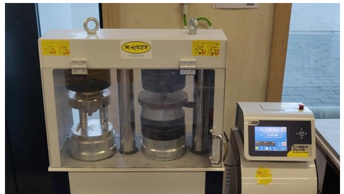
Figure 6: MacBen compression test for mechanical characterisation.
