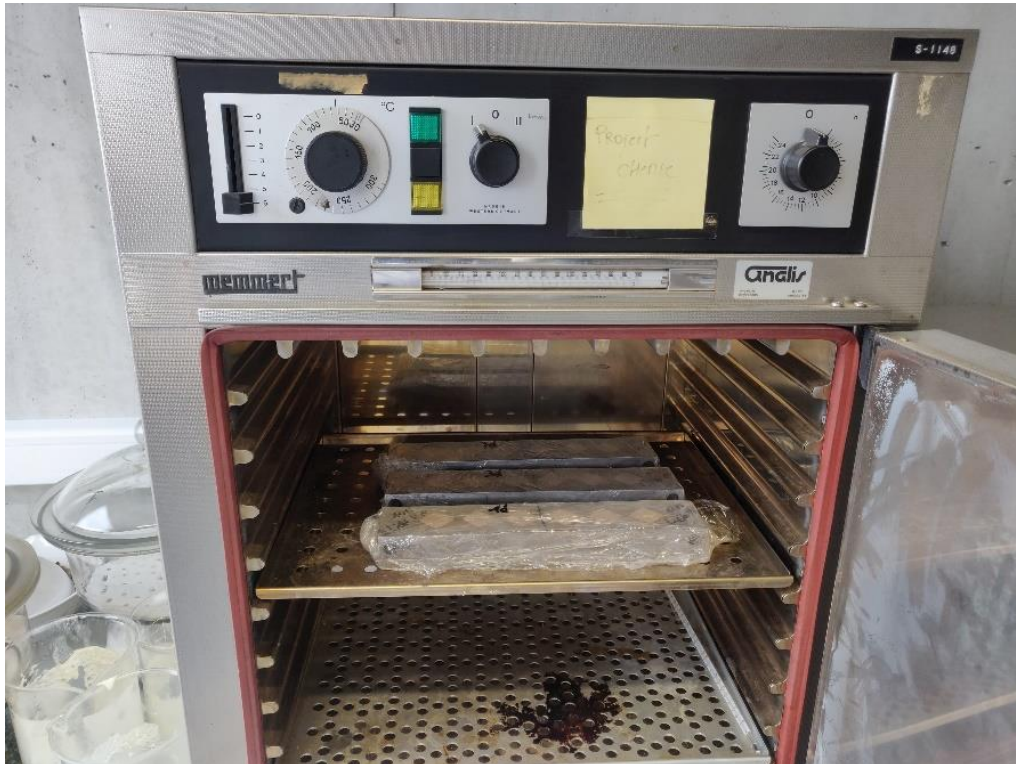
Figure 56: Oven at 70 °C for curing process of geopolymers.
