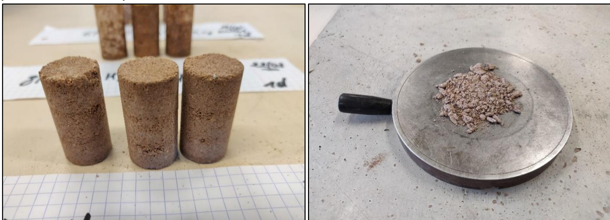
Figure 119: 8M NaOH-based cylindrical geopolymers before (left) and after compression test (right).
