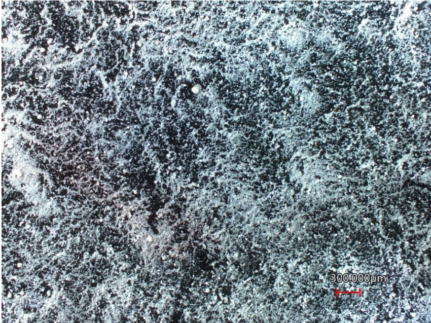
Figure 111: Metakaolin after calcination for 3 hours at 650 ^{\circ}\text{C} – scale bar 300 \mu\text{m} .
