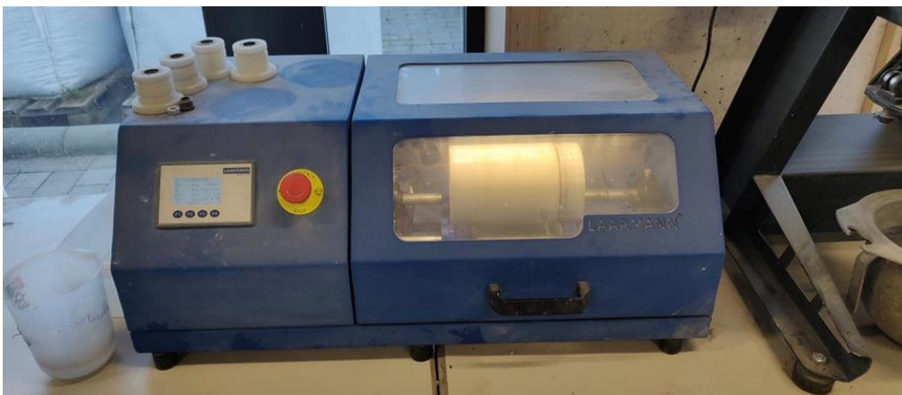
Figure 78: LMBR500 Bottle Roller for grinding the MGS-1 simulant.
