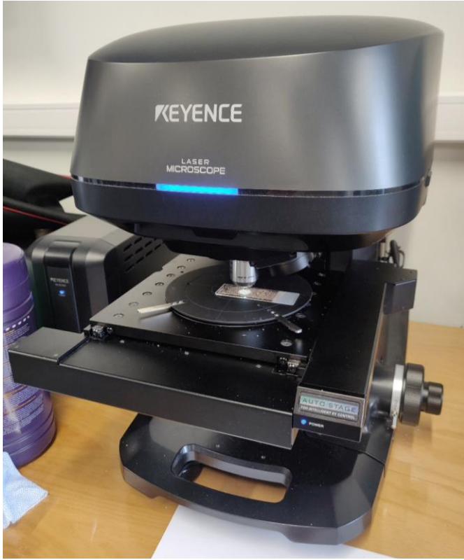
Figure 7: Keyence laser microscope for determining the effect of grinding MGS-1 and calcination of kaolinite.
