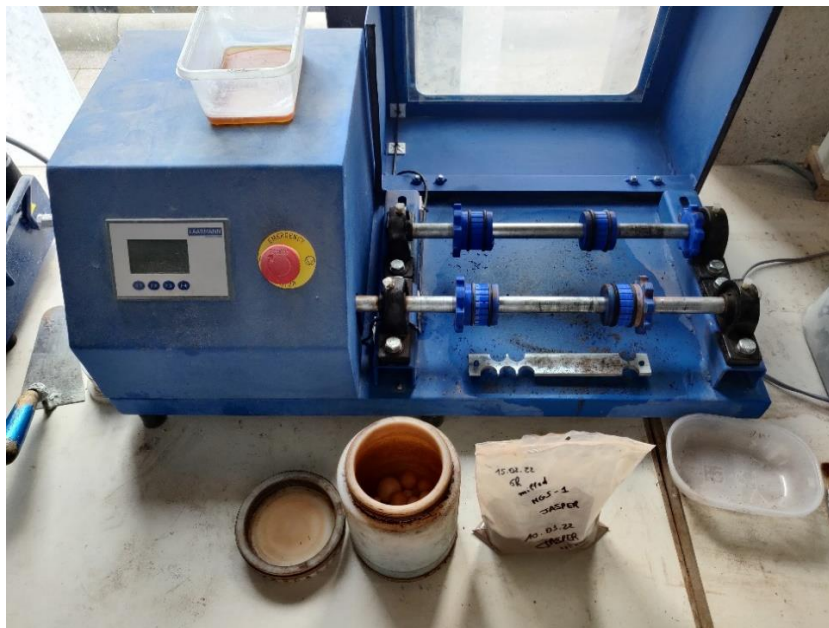
Figure 62: Bottle Roller for grinding the MGS-1 simulant.
