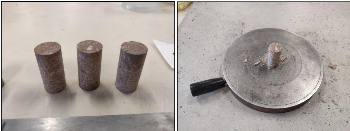
Figure 121: 8M LiOH.H 2 O + 7.5 g NaOH-based cylindrical geopolymers before (left) and after compression test (right).
