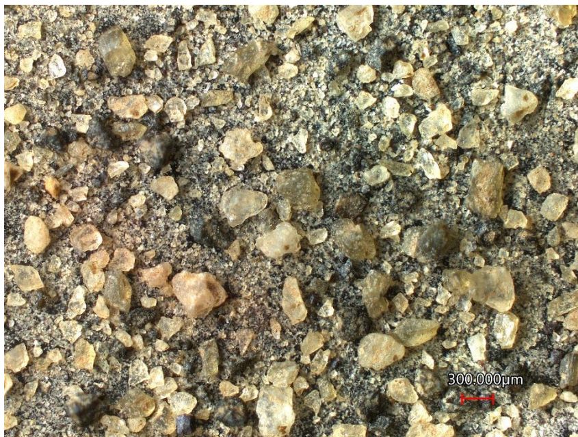
Figure 107: MGS-1 after grinding for 6 hours by Bottle Roller – scale bar 300 \mu\text{m} .
