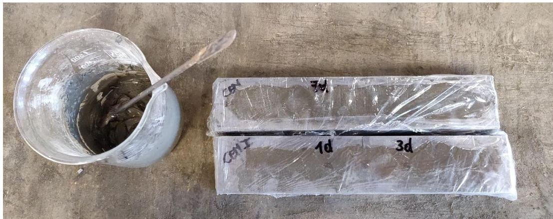
Figure 66: Portland cement CEM I 52.5R HES cube samples.
