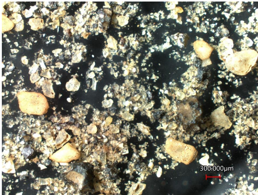
Figure 106: MGS-1 before grinding – scale bar 300 \mu\text{m} .
