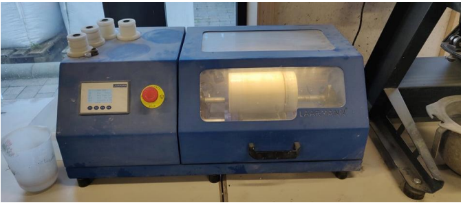
Figure 4: LMBR 500 Bottle Roller for grinding the MGS-1.
