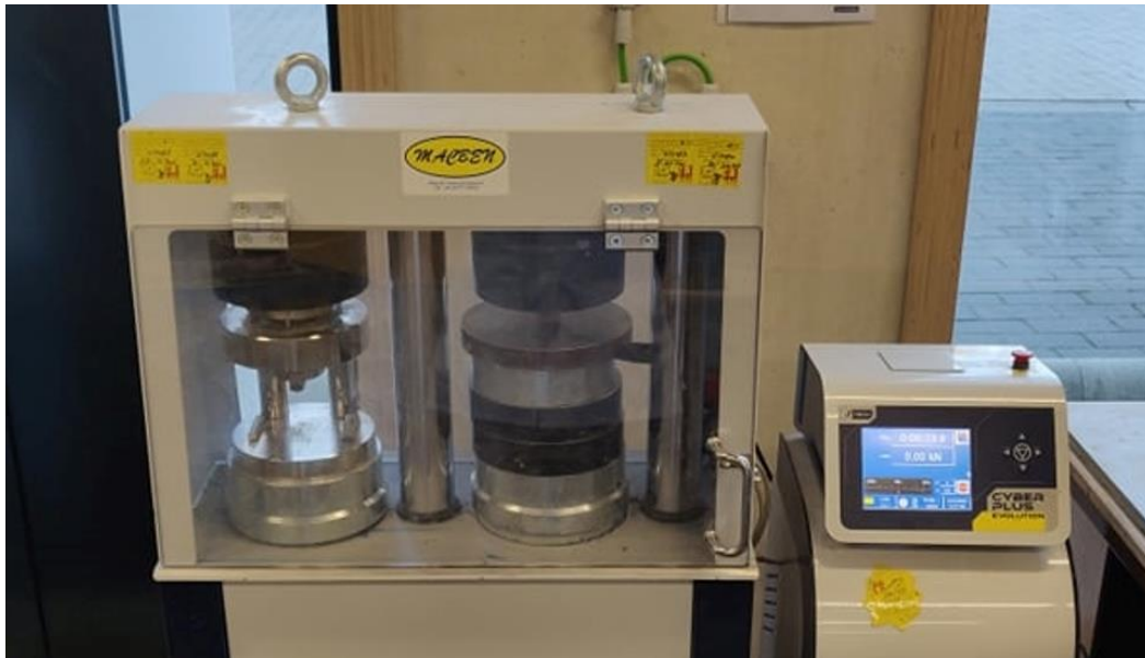
Figure 77: MacBen compression test for mechanical characterisation.
