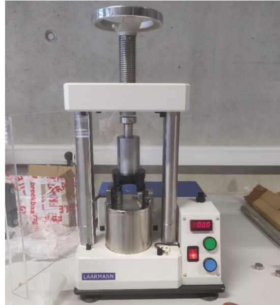
Figure 3: Pellet press for compaction of cylindrical geopolymer samples.
