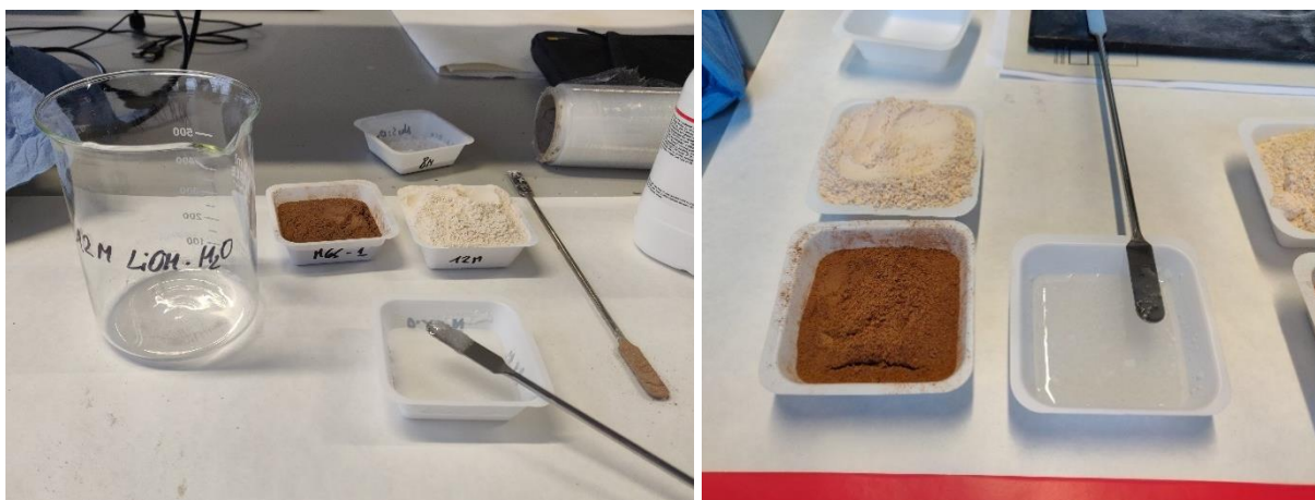
Figure 72: Increased solubility of \text{LiOH} \cdot \text{H}_2\text{O} in \text{Na}_2\text{SiO}_3 solution by 5 g NaOH pellets catalysation.
