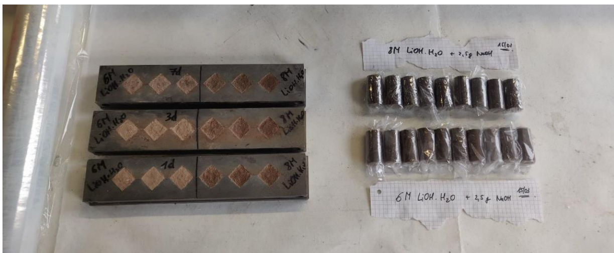
Figure 64: Cube (left) and cylindrical (right) geopolymer samples, before curing.
