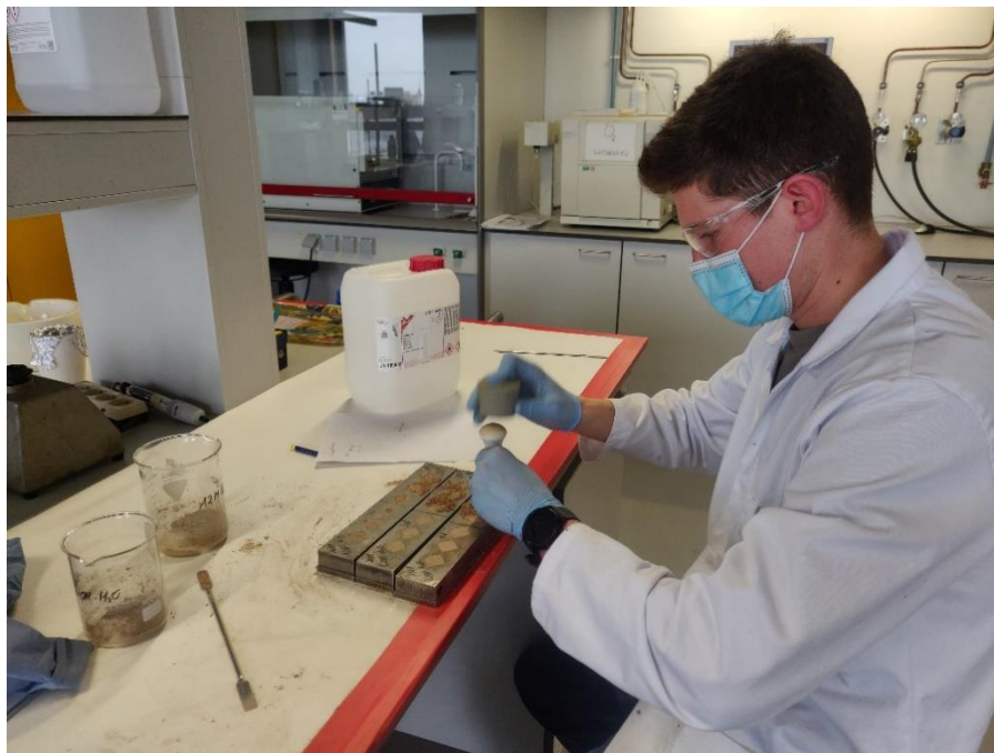
Figure 61: Manual compaction of the cube geopolymer samples during research work.
