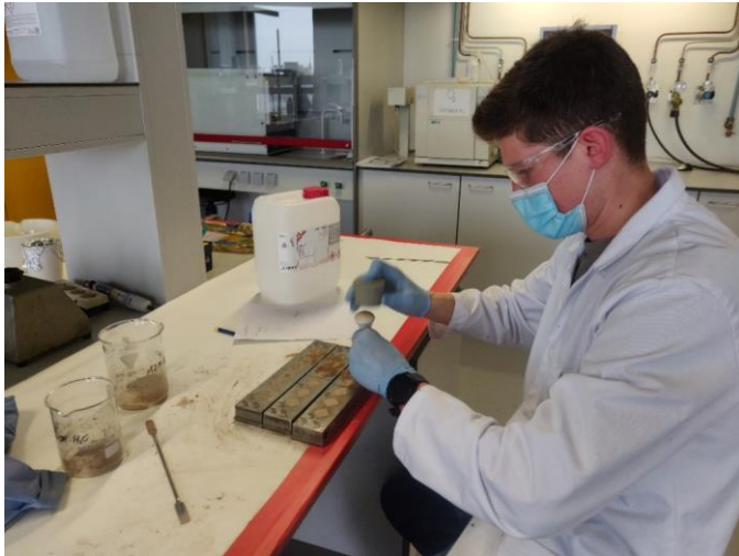
Figure 2: Manual compaction of cube geopolymer samples.
