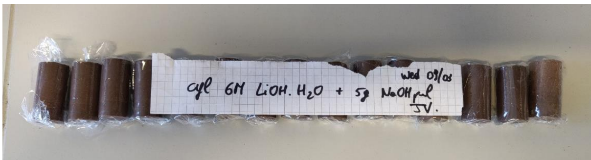
Figure 57: Cylindrical geopolymer samples of 6M LiOH. H 2 O + 5 g NaOH.
