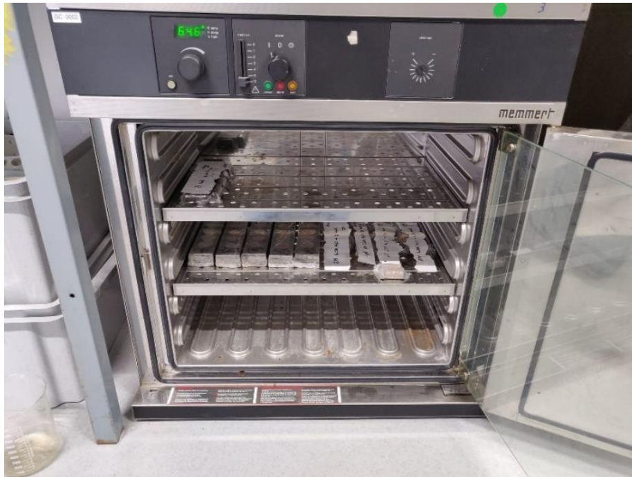
Figure 63: Cube and cylindrical geopolymer samples in oven at curing temperature of 70 °C.
