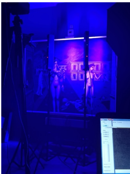
Figure 31: Set-up of the UV-VIS HIS by the Perugia team.
