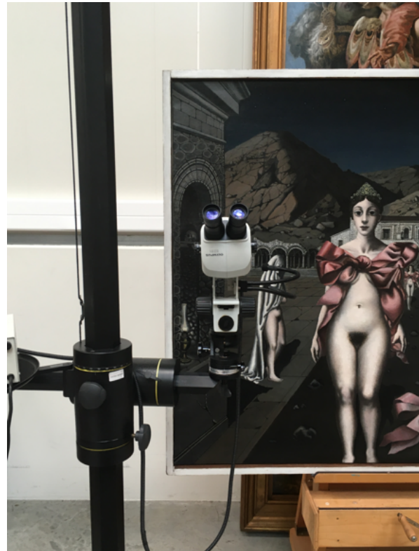
Figure 24: Stereo microscope mounted on a tripod.
