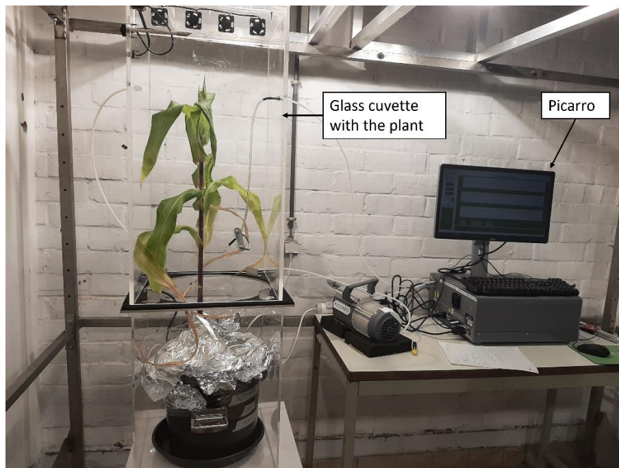
Figure S.2: Set-up ^{13}\text{C} labelling. The plant (experiment 1 treatment P+AMF+) was placed in the glass cuvette for labelling with ^{13}\text{CO}_2 . To measure the ^{12}\text{CO}_2 and ^{13}\text{CO}_2 concentrations in the cuvette, a Picarro was connected. The soil of the plant was covered by aluminium in order to avoid take up of ^{13}\text{CO}_2 by soil bacteria.
