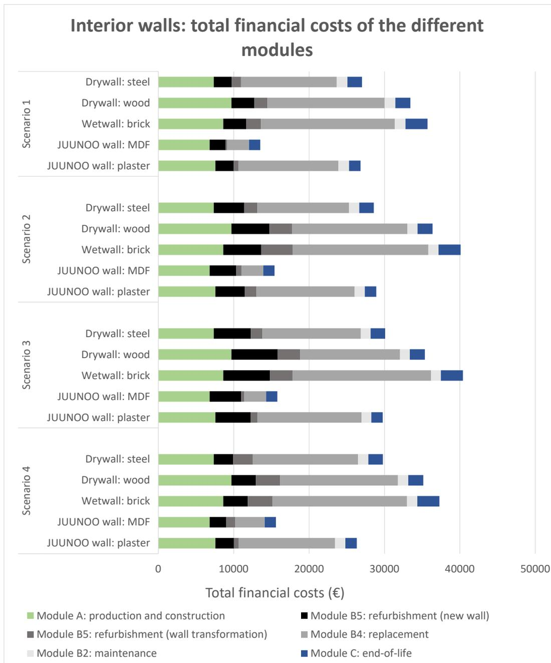
Figure 6.22: Overview of the financial costs of the different modules: production, construction, use and end-of-life stage, for the different interior walls for the four refurbishment scenarios.
