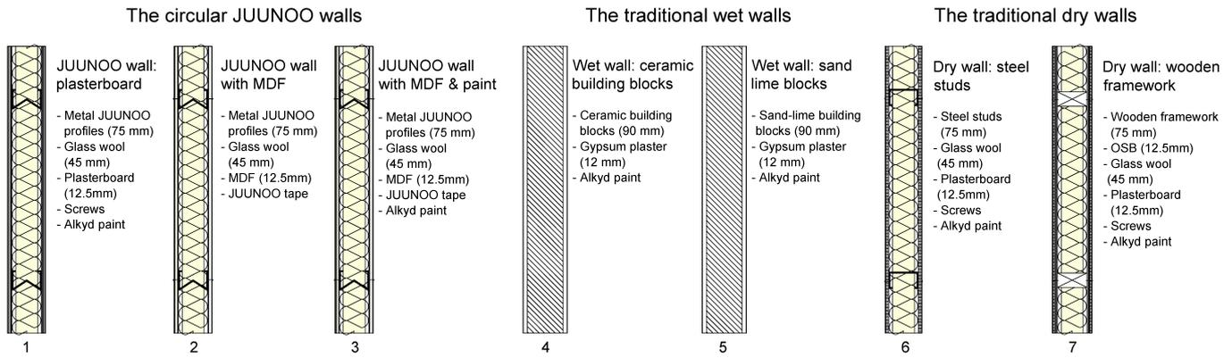
Fig. 2. The seven investigated interior walls in the case house in Berchem.
