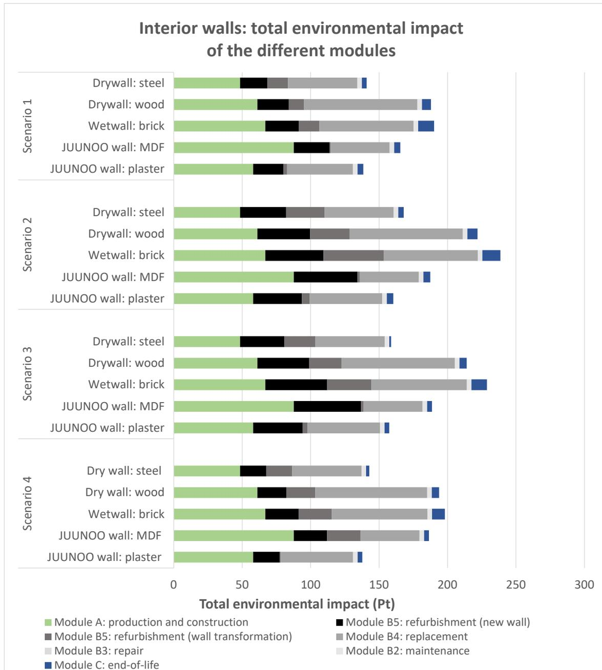
Figure 6.20: Overview of the environmental impacts of the different modules: production, construction, use and end-of-life stage, for the different interior walls for the four refurbishment scenarios.
