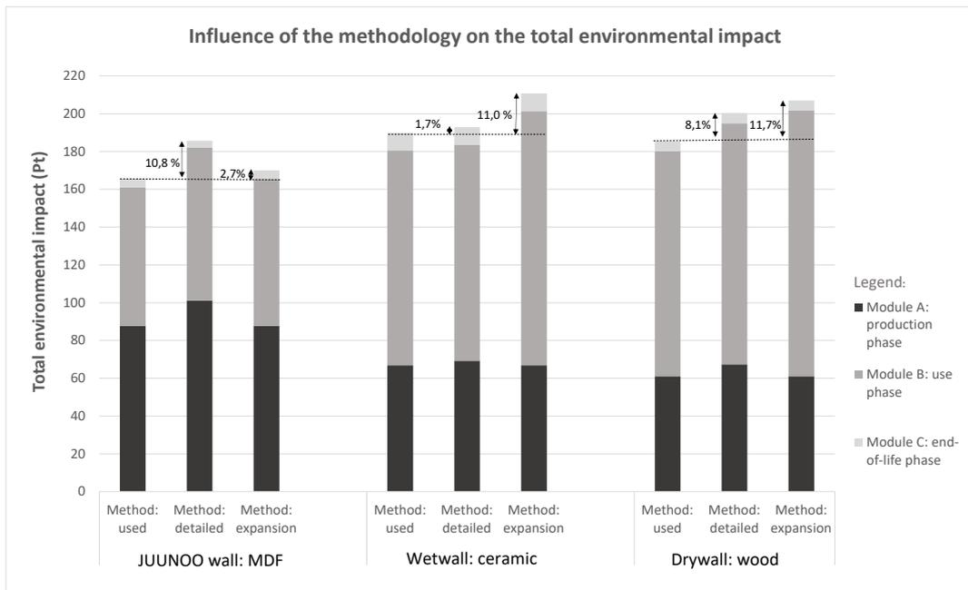
Figure 6.25: Sensitivity analysis on the total environmental impact of the wetwall with ceramic bricks, the drywall with wooden frame and the JUUNOO wall with MDF, calculated with the used, expanded and detailed method for scenario 1.
