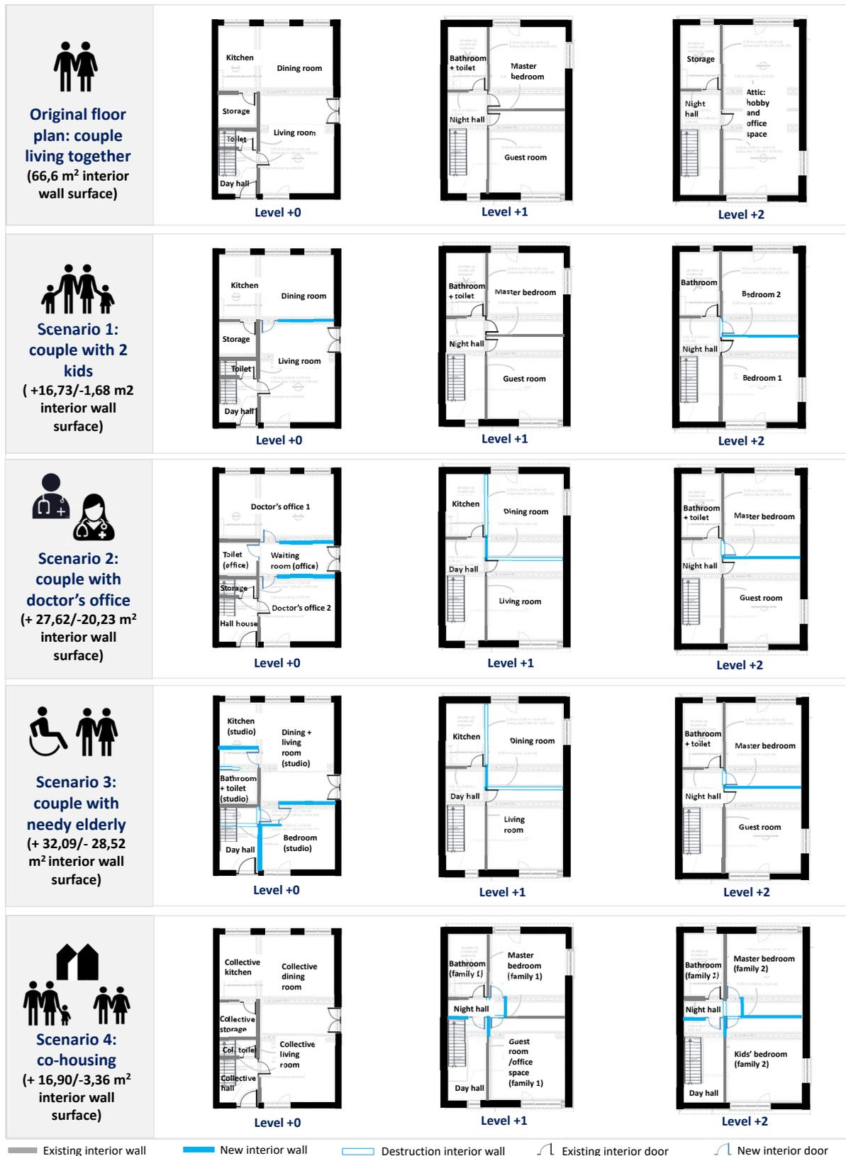
Figure 6.17: Overview of the original floor plan and the floor plans of the four refurbishment scenarios with the transformed walls.
