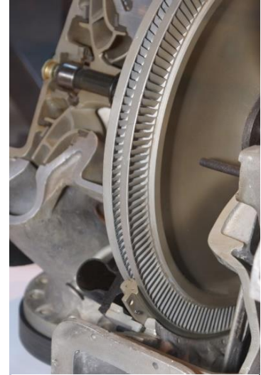
Figuur 19 V2 steam turbine rotor https://v2rockethistory.com/turbo-pump-parts-and-relics/
