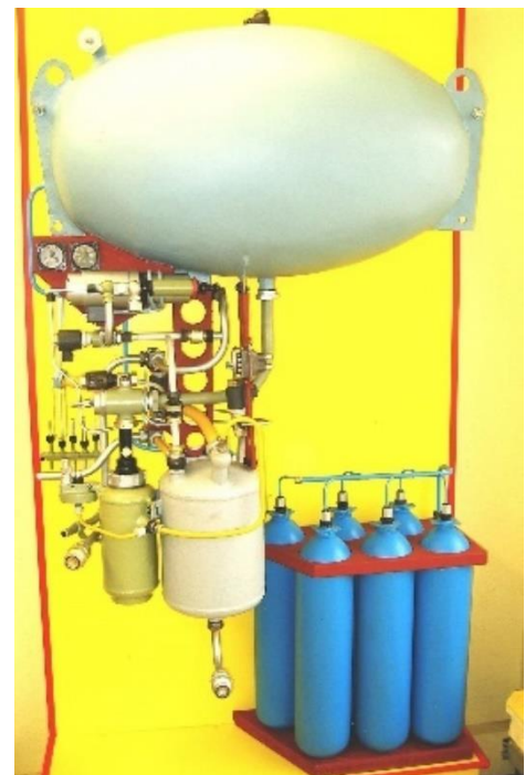
Figuur 22 V2 gas generator https://v2rockethistory.com/gmedia/a4-v2-missile-steam-plant-detail-jpg/
