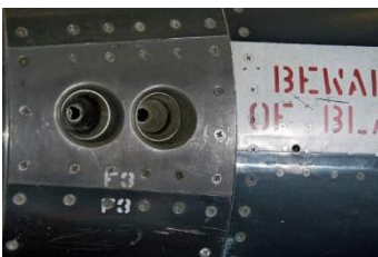
Figuur 27 RCS, https://space.stackexchange.com
