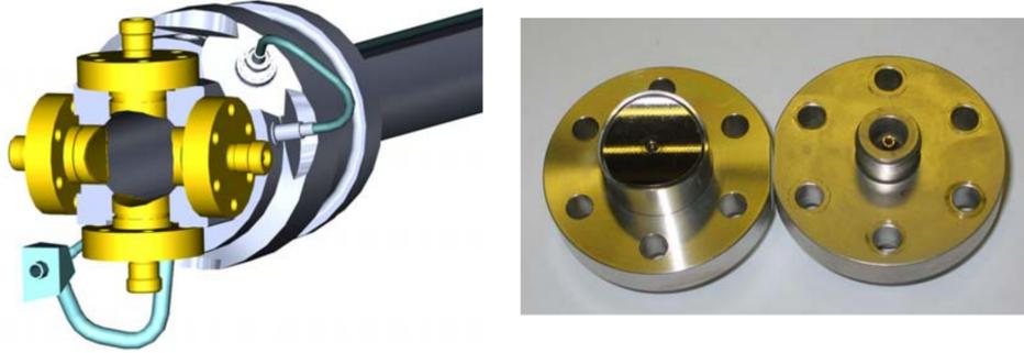
**Fig. 2.3.:** **Left:** schematic drawing of a button BPM configuration. **Right:** parts of a button BPM used at LHC. The left part is directed towards the inside of the beam tube. Images from [60].
