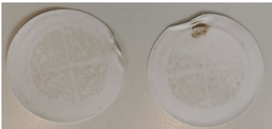
Figure 16: The sediment particles on the filters after the two MFI tests were carried out.
