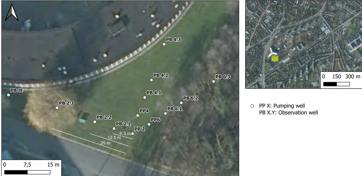
Figure 4: Localization of the well area used for pumping tests on Campus Sterre.
