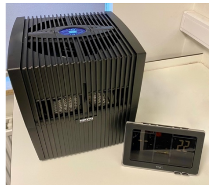
Figure 2. Setup of the room humidifier and thermometer. The room temperature was kept at 22°C with a relative humidity of around 55%.
