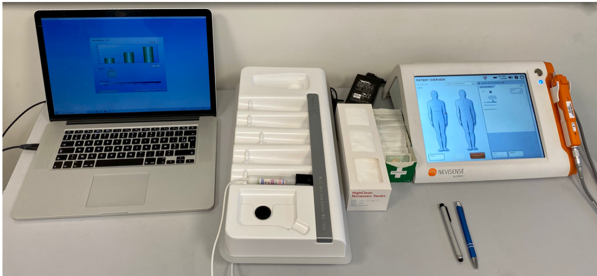
Figure 6. Overview of the study setup. Set up of the Multi Skin Test Center MC 1000 open-chamber device (left) connected to a laptop and the Nevisense system (right).
