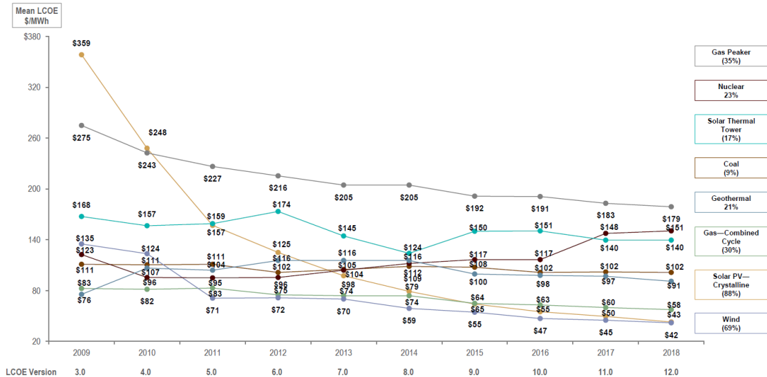
Figure 1.5: Historical evolution of the unsubsidized Levelized Cost Of Electricity ($/MWh) for the main energy generation sources [10]. Renewable energies are now cost competitive.
