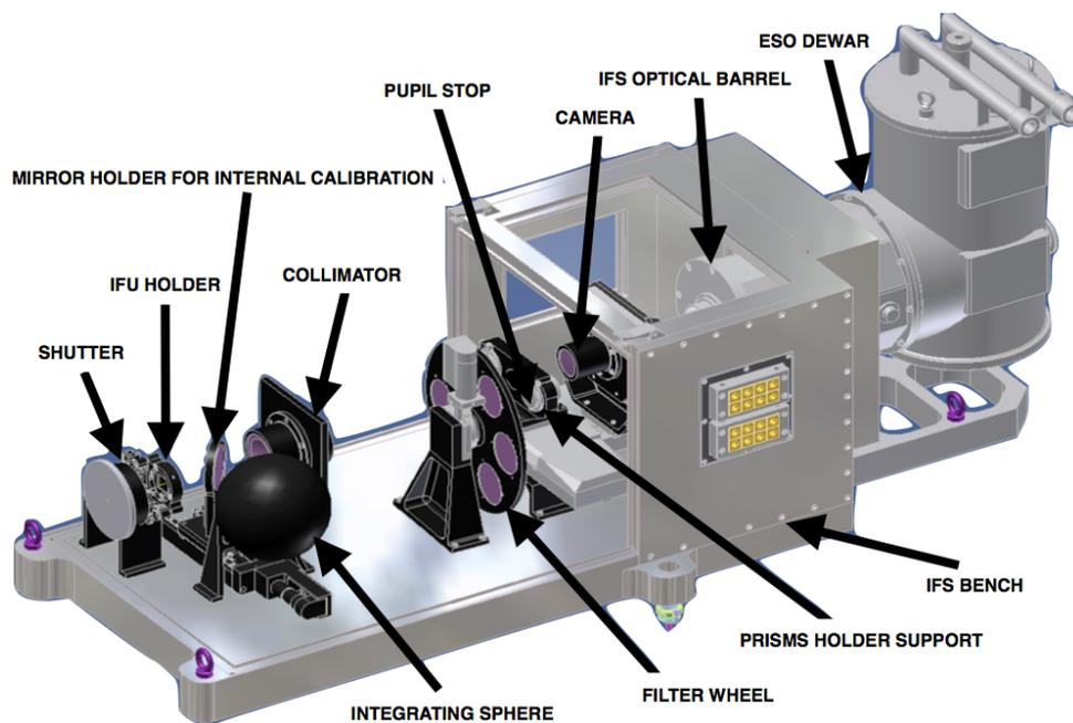
Figure 2.2: Diagram of the Integral Field Spectrograph (IFS) on SPHERE. Figure Credit: [European Southern Observatory, 2021b]
