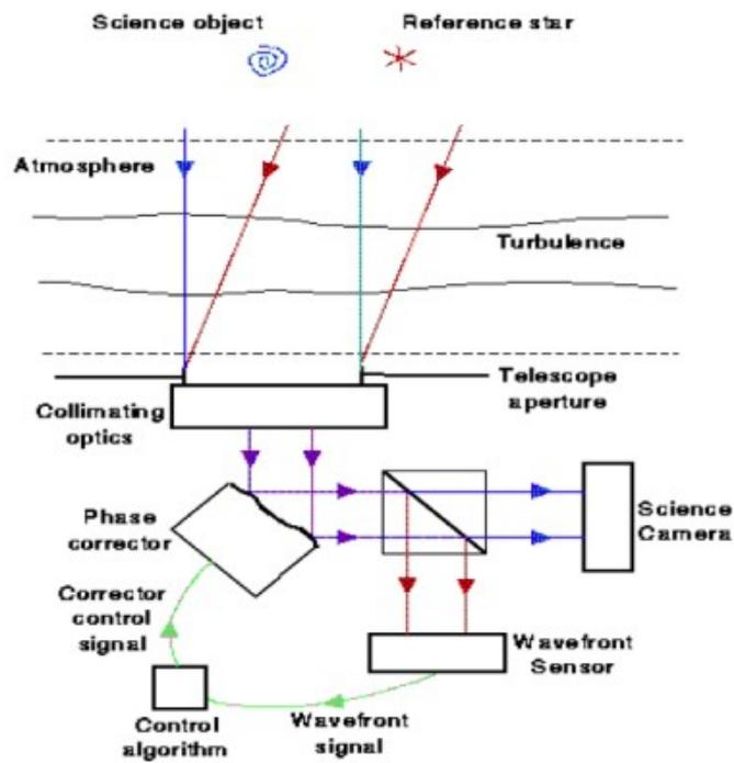
Figure 2.4: Block diagram of a simple AO system. Light from a reference source, such as a star, bounces off a deformable mirror and a portion enters a wavefront sensor. This control system generates a correction signal which moves the deformable mirror, reducing the error. The light leaving the deformable mirror is refocused onto a detector or science camera. Figure Credit: David Carter, Liverpool John Mores University [Carrasco, 2009].
