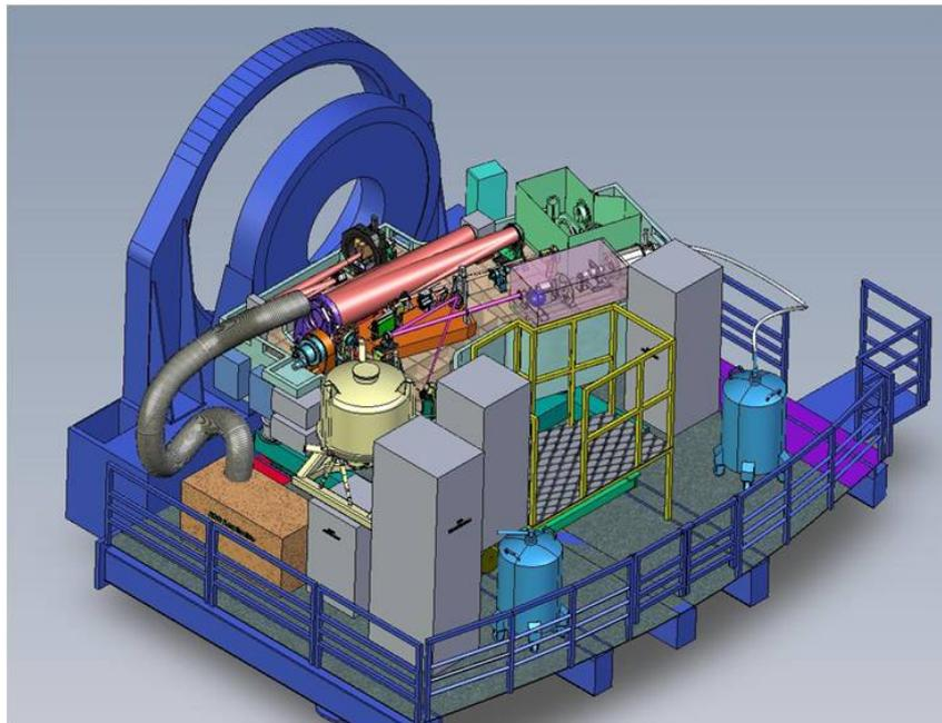
Figure 2.1: Diagram of the Spectro-Polarimetric High-contrast Exoplanet REsearch (SPHERE). Figure Credit: [European Southern Observatory, 2021b]
