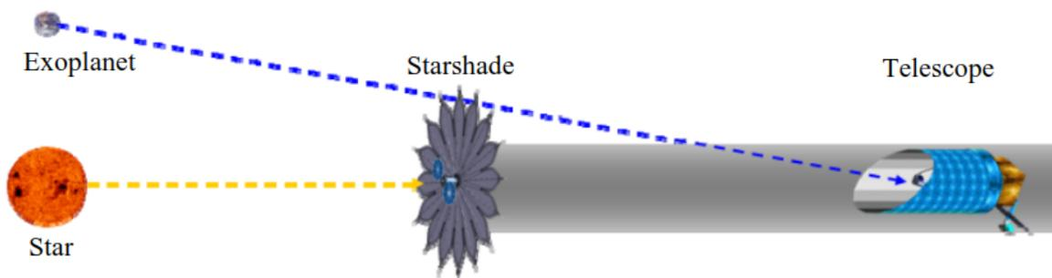
Figure 5.3: A diagram of a star shade. The (unlabeled) details of the figure (i.e., telescope diameter, starshade diameter, telescope-starshade separation, planet-star separation or "inner working angle", wavelength sensitivity range, etc.) will determine what kind of planets will be detectable by the system. Figure Credit: Glassman et al. [2009]
