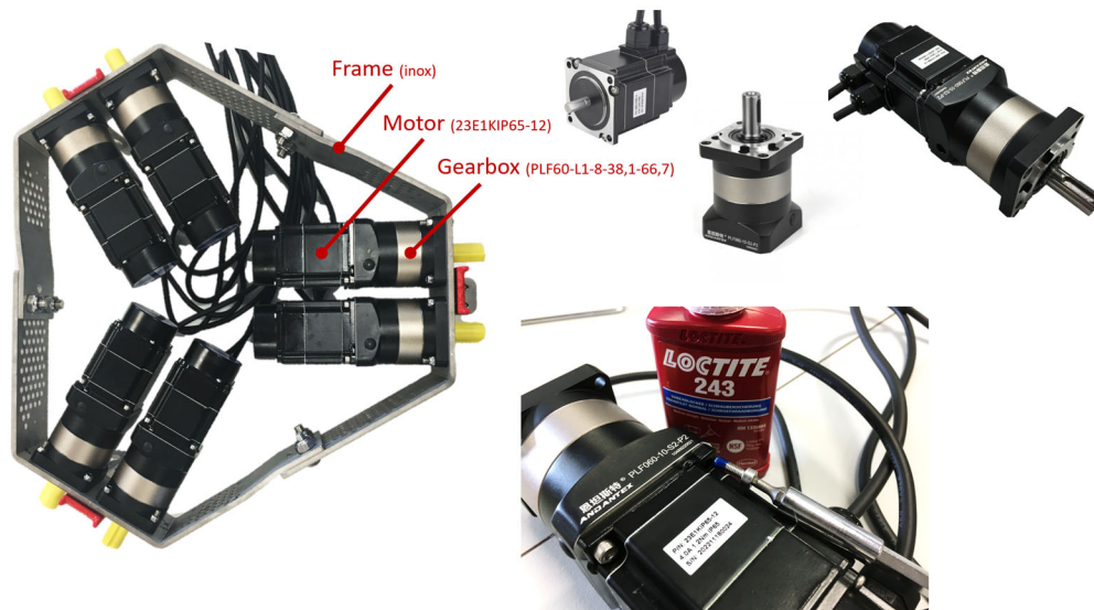
Figuur 57: Assemblage motor, transmissie en frame | Noot: copyright 2023 Bram Dupré
