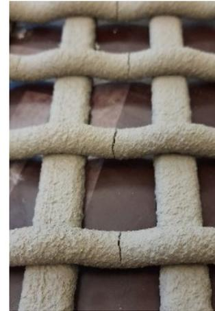
Figure 4.5. Cracking occurs in the concrete at the weakest points, caused by drying shrinkage and increasing inner stresses.
