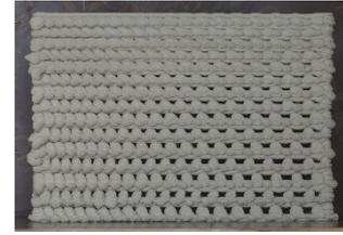
*Figure 4.47.* Alternating *Greek Key Pattern* creates a staggered arrangement.
