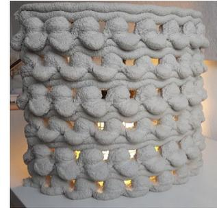
Figure 4.43. Arc shaped panel shows rough texture and perforations that transmit light.
