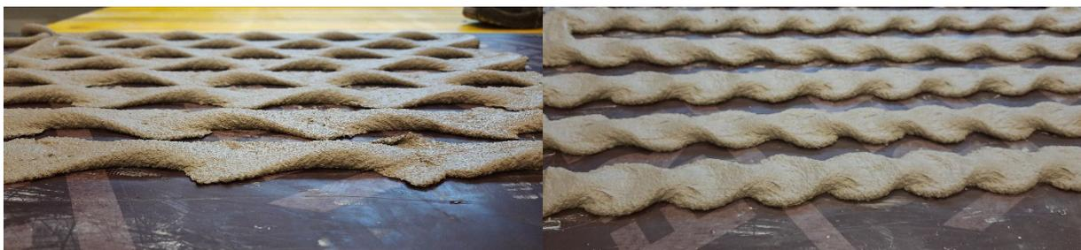
Figure 4.15. Printed results of the vertical zig-zag line. Left) first attempt shows cladding on the sides, right) Vertical zig-zag line, whole geometry moved 2mm up.
