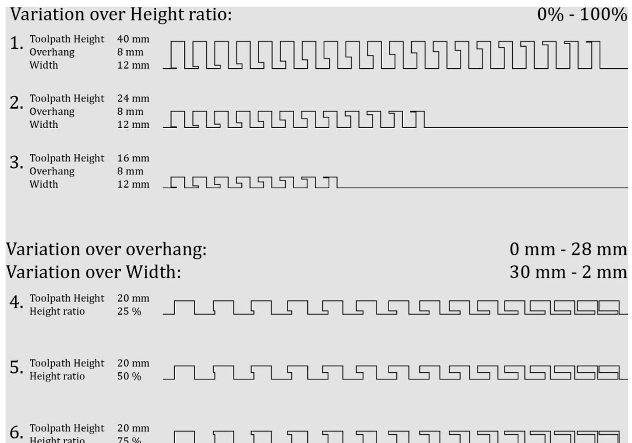
Figure 4.29. Used toolpaths and parameters for iterative parameterisation of the *Greek Key Shape*.
