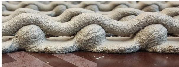
Figure 4.40. Z-height of straight line influences the perforation area of the *Greek Key*.
