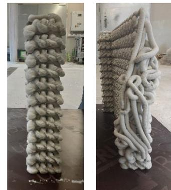
Figure 4.50. Greek Key based support: left side shows cumulative failure, right side provides support.
