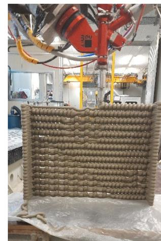
Figure 4.58. A plastic foil on top of the last lines of the previous panel is used to leave an imprint in the new printed panel.
