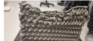
*Figure 4.48.* Double straight layer leads to failure of the panel.
