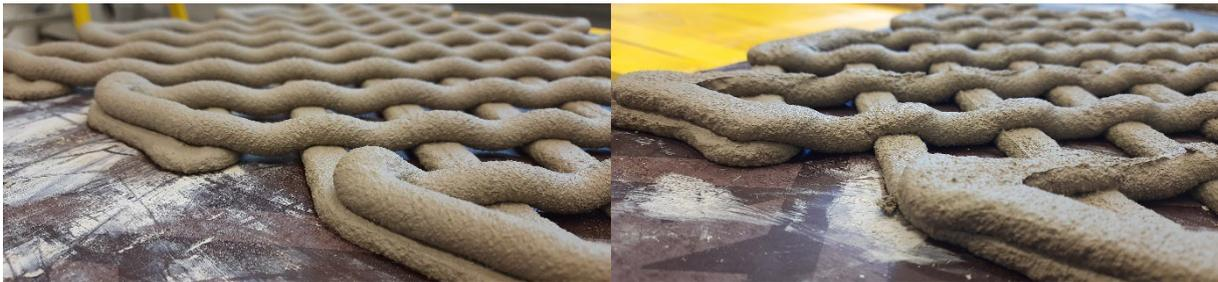
Figure 4.9. A higher layer height (left) results in a rounder cross-section but a weaker intermixing between layers. Layer height of 8mm (right) provides a strong intermixing between layers.
