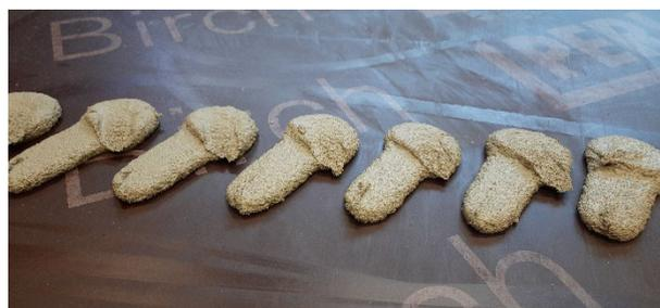
Figure 4.18. Printed result of a line, made with the pinch valve.
