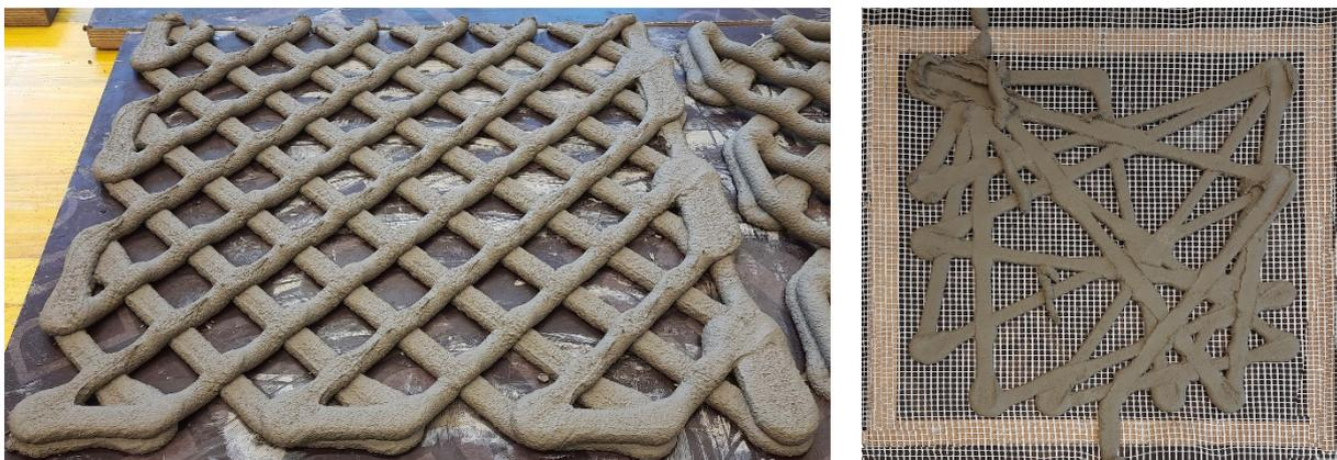
Figure 4.4. Printed results of left) Horizontal Diagonal Grid, right) Horizontal Glass Optic Fibre Network Panel showing the opportunities and challenges of creating a horizontal perforated panel with a 3D concrete printer.
