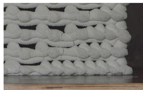
Figure 4.59. Panel was not covered with a plastic foil during the hardening process, which has led to cracking.
