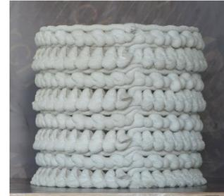
*Figure 4.61.* A seam is visible on a closed surface because the printer moves up from one layer to the next.
