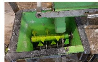
Figure 3.5. A worm screw in the mortar pump rotates and pushes the concrete towards the print nozzle.
