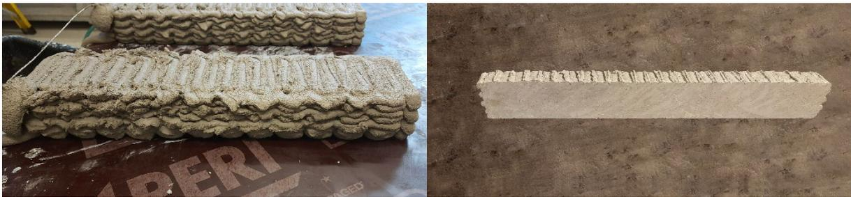
Figure 4.21. Printed result of glass optic fibre panel.
