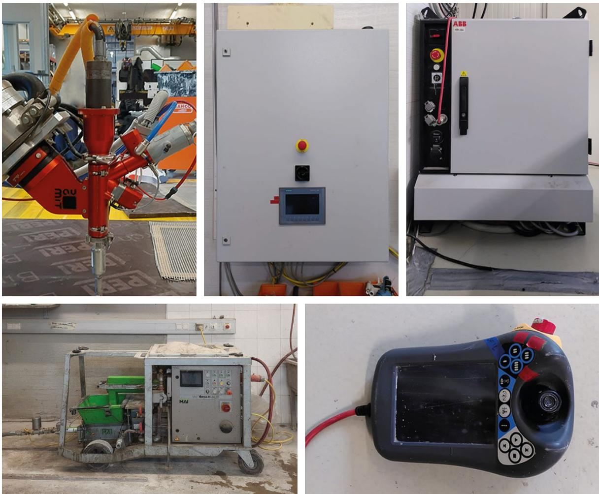
Figure 3.3. Different components of the 3D concrete printer setup at TU Graz. From left to right, top to bottom: BauMinator print nozzle, PLC, KCU, Mortar pump and Kinematics controller.
