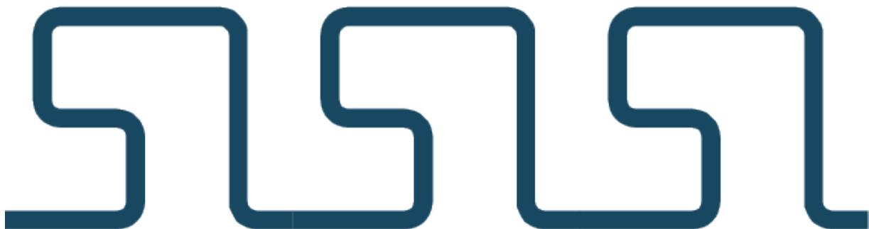
Figure 4.23. Toolpath followed by the 3D concrete printer, to fabricate a *Greek Key Line*.
