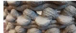
Figure 4.44. Alternating pattern between *Greek Key* and hanging slab fabricates a rough texture.
