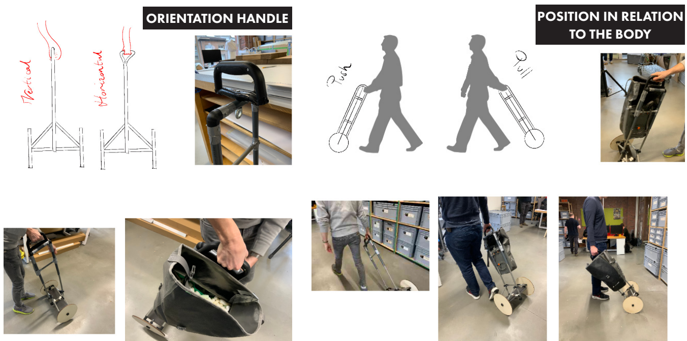
Figure 88 - prototyping and testing different ergonomics of the handle (left) and positioning (right)
