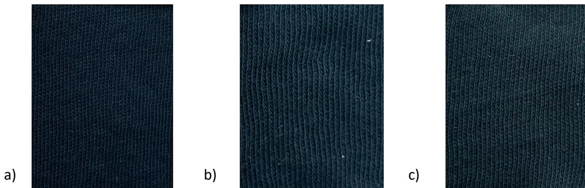
Figure A.5: black-dyed cotton before (a) and after Fenton-treatment with FeSO<sub>4</sub> (b) and FeCl<sub>3</sub> (c).
