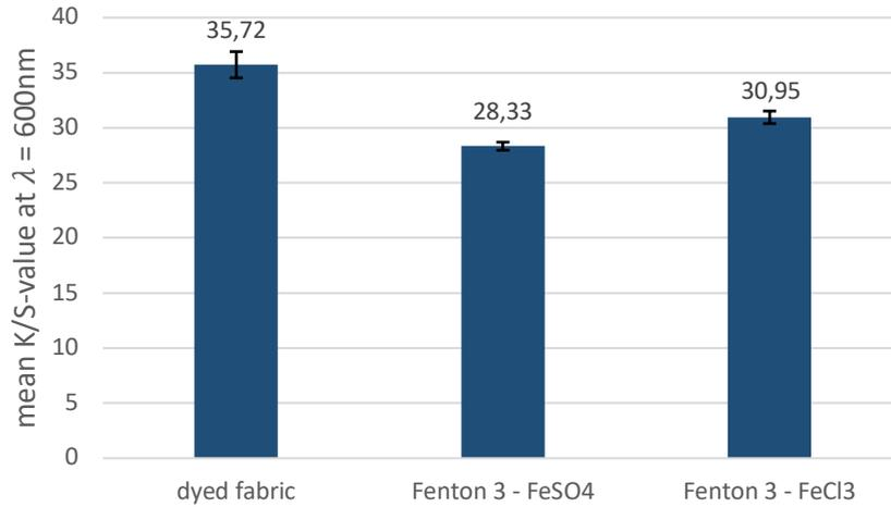
Graph A.4: mean K/S-values of the black-dyed cotton before and after Fenton treatments with different iron-sources (FeSO<sub>4</sub>x7H<sub>2</sub>O and FeCl<sub>3</sub>).
