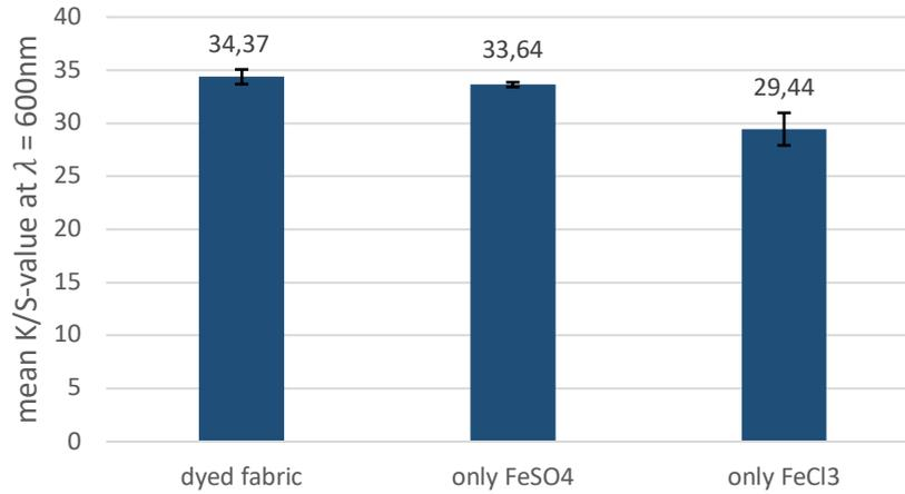
Graph A.9: mean K/S-values of the black-dyed cotton before and after treatments with only the iron-sources FeSO<sub>4</sub>x7H<sub>2</sub>O and FeCl<sub>3</sub> (without H<sub>2</sub>O<sub>2</sub>).
