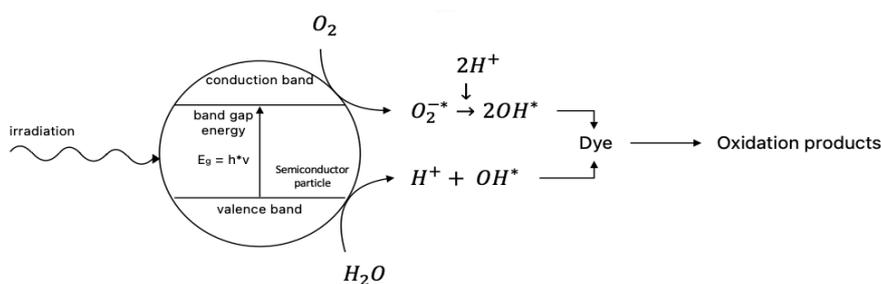
Figure 2.5: mechanisms occurring in photocatalytic dye-degradation: catalyzed by a semiconductor particle and initiated by irradiation of a light-energy source, based on Ajmal et al. (2014).
