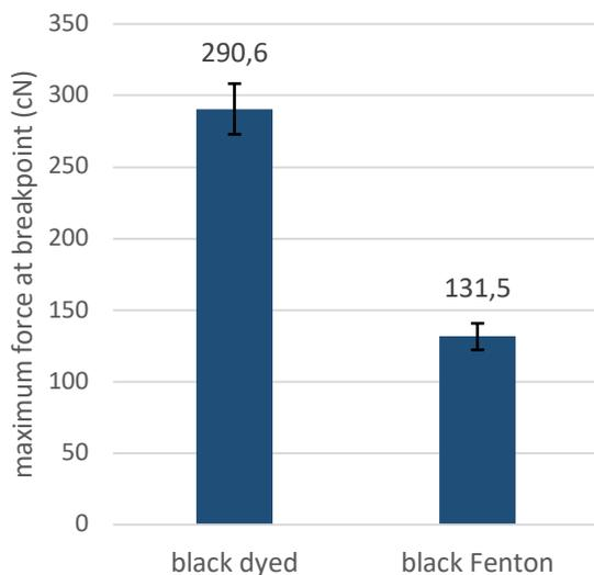
Graph 4.12: mean values of maximum force at breakpoint of the raw cotton, black-dyed cotton and Fenton-treated cotton, measured during tensile testing of the unraveled yarn.
