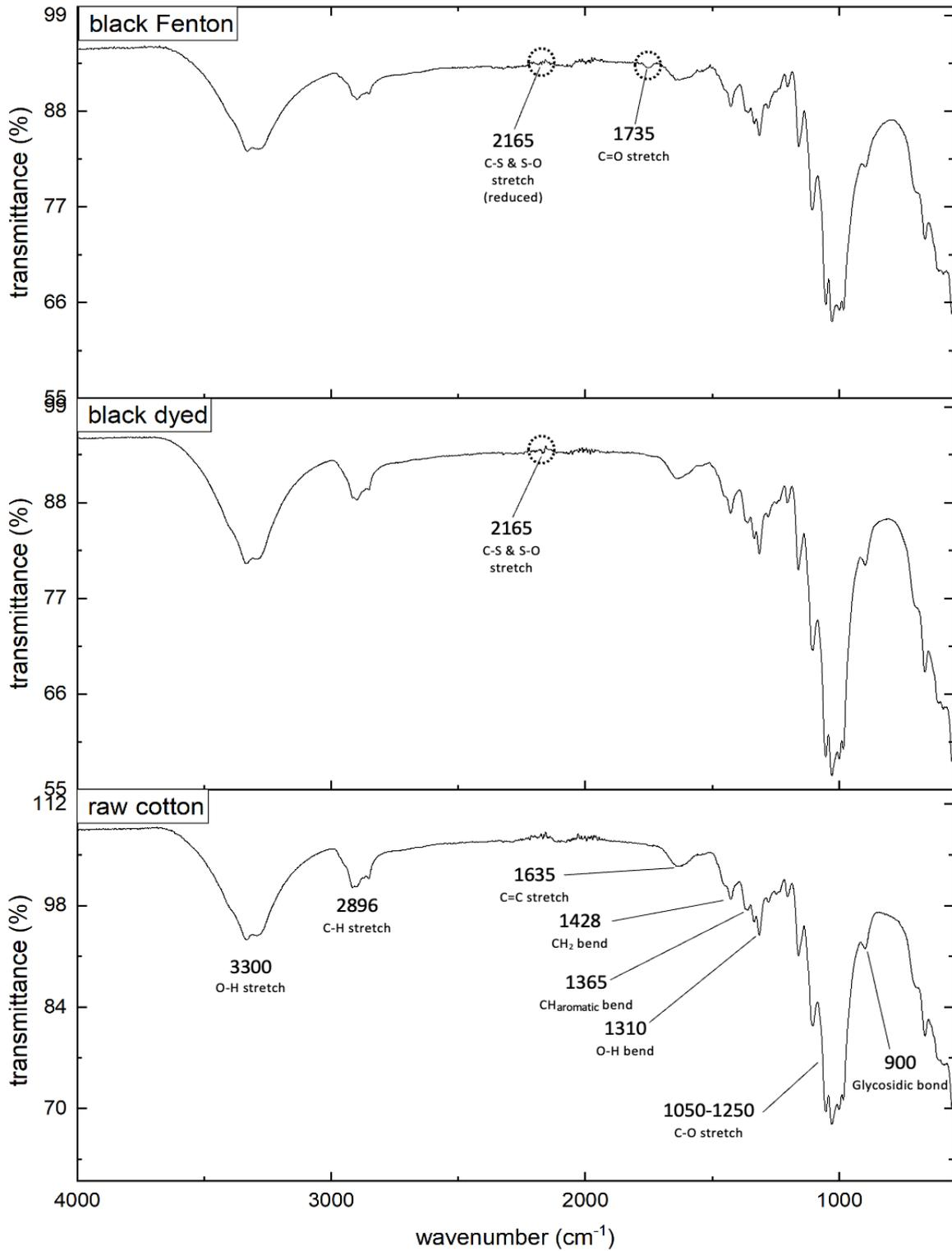
Graph 4.10: Stacked FTIR -spectra (transmittance % versus wavenumber) of raw cotton, black-dyed cotton and black Fenton-discolored cotton.
