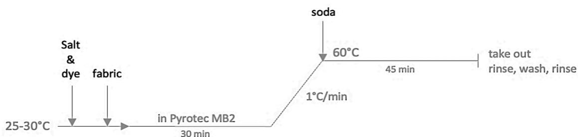
Figure 3.1: graphical representation of the applied dyeing process.
