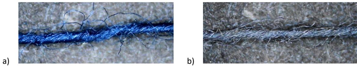
Figure 4.6: microscope-images of black-dyed cotton yarns before (a) and after (b) Fenton-treatment.
