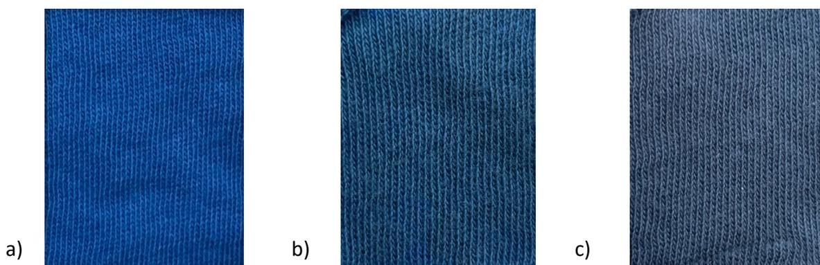
Figure A.7: black-dyed cotton before (a) and after Fenton-treatment with FeSO<sub>4</sub> (b) and FeCl<sub>3</sub> (c).
