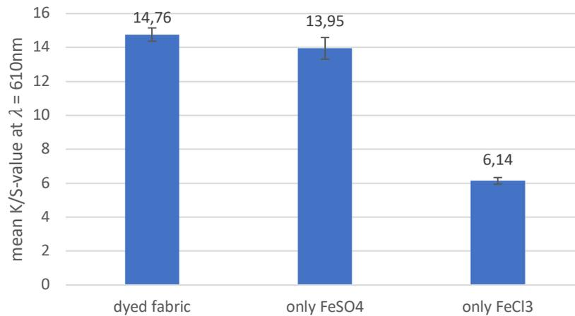
Figure A.10: mean K/S-values of the blue-dyed cotton before and after treatments with only the iron-sources FeSO<sub>4</sub>x7H<sub>2</sub>O and FeCl<sub>3</sub> (without H<sub>2</sub>O<sub>2</sub>).
