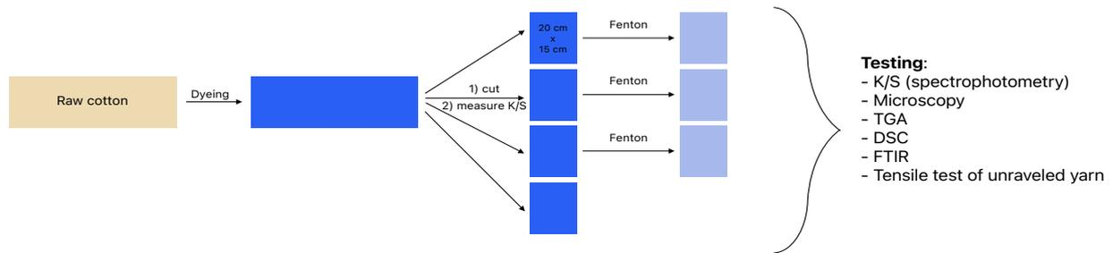
Figure 3.2: visual representation of the plan for Fenton-upscaling and further analysis.
