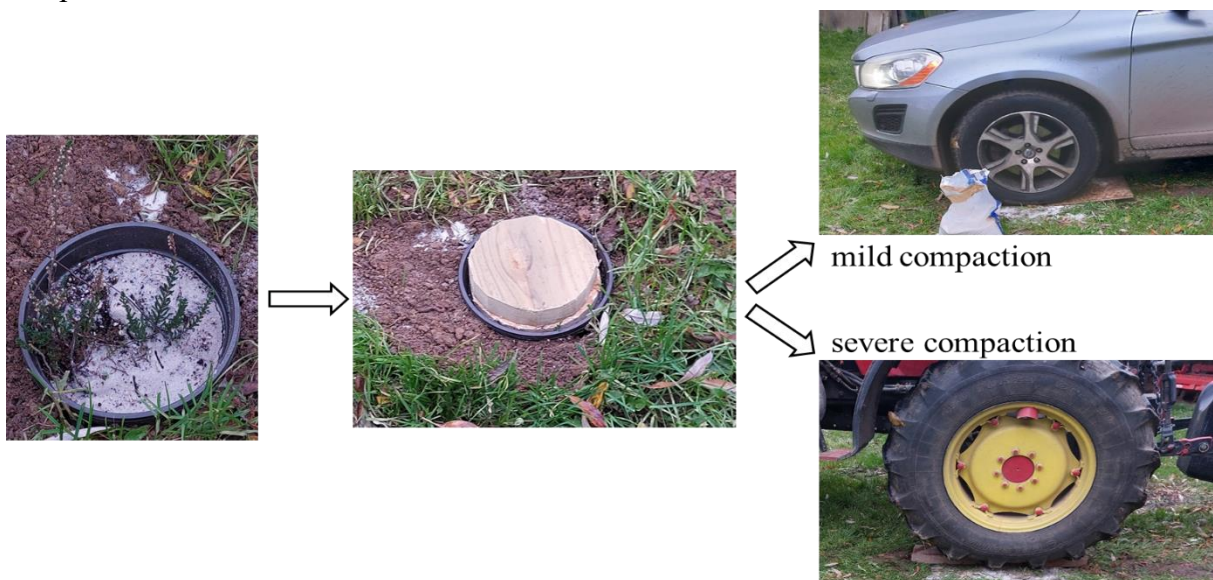
Figure 4: Setup for experimental compaction of the soil in the ‘mild’ and ‘severe compaction’ treatments. See main text for a detailed explanation.
