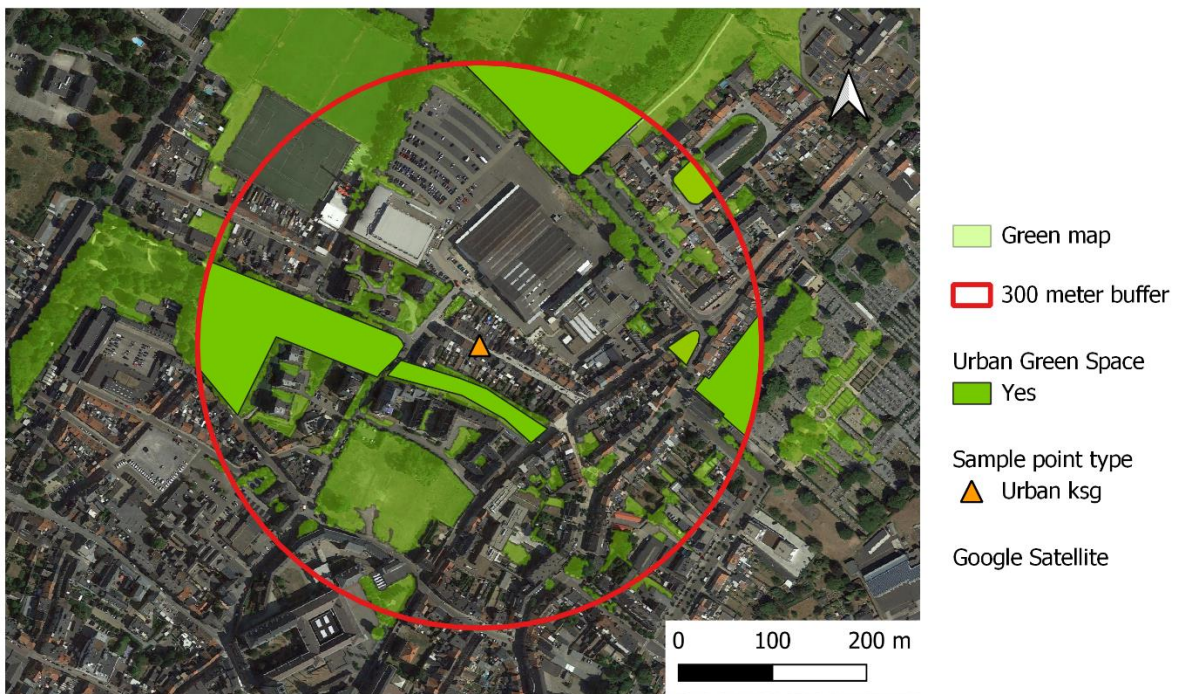
Figure 8.4: Example sample point 38 with green map created based on land cover map (Agentschap Digitaal Vlaanderen, 2021). A 300 m buffer around the sample point is indicated. The sample point type is urban ksg (which stands for 'kleinstedelijk gebied', meaning small urban area). The delineated Urban Green Spaces are indicated as well.
