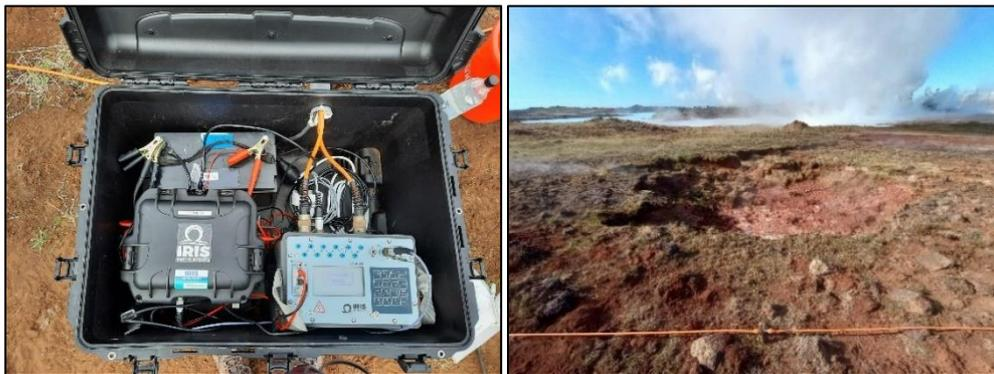
Figure 7: the box with ERT measuring equipment during the field campaign and the ERT electrode connected to the cable on the field; for the monitoring study, an extra battery and charger are present in the box
