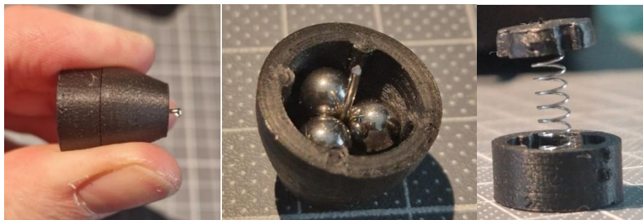
Figure 48: Test 4 shell (left), inside (middle) and spring (right)(own figure)
