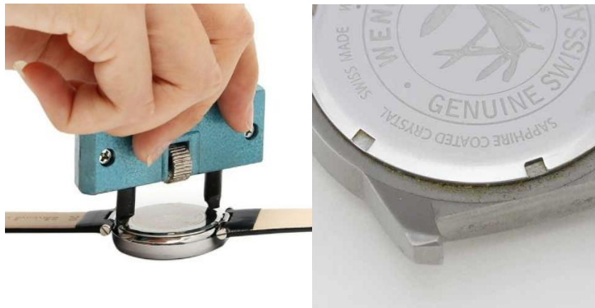
Figure 55: Watch back with notches [69] (left) and watch back removal tool [70] (right)
