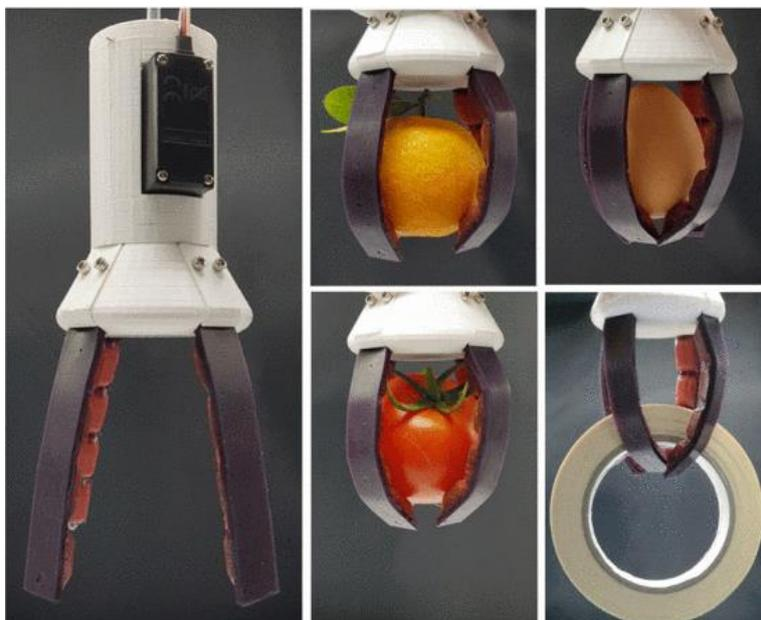
Figure 3 An example of a tendon driven actuator used for a gripper grasping multiple objects [22]
