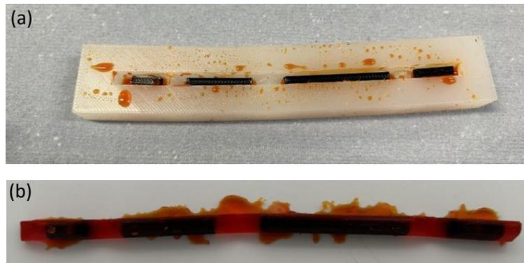
Figure 34 (a) The mould prepared to cast half of the actuator and (b) the result of this casting.
