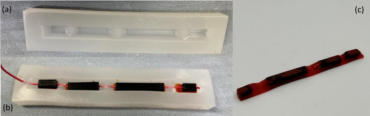
Figure 32 An actuator being manufactures using multi-stage casting. (a) shows the used mould, (b) shows the mould before the second casting step where it can be observed that the rigid parts are placed on the already cast material and (c) shows the final result.
