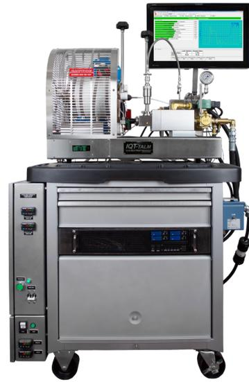
(b) Totally Automated Laboratory Model of a Ignition Quality Tester apparatus [58].
