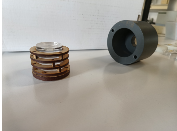
(b) The sources in the wooden holders and the lead cylinder
