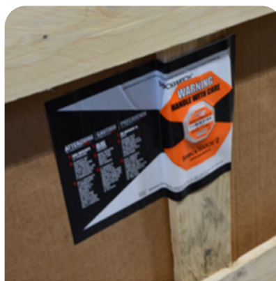
Figuur 1.39: Shock & tilt watch 1
