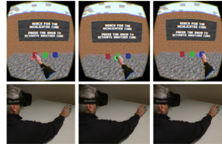
(b) 1 for 3 Illusion - User touches 3 different virtual cubes while in reality the same cube is touched each time[Azm+16].
