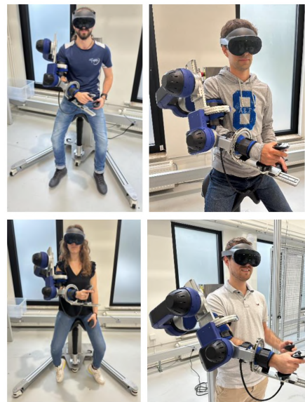
(d) Integrated X-aRm system with different candidates validating comfort, adjustability and portability[Bar+23].
