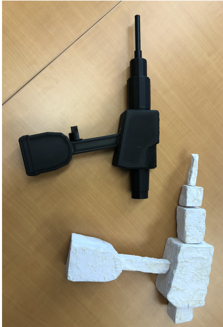
Figure 4.12: The 3D printed PGT at the top left and the styrofoam PGT at the bottom right. The 3D printed PGT includes a slide and lock magnet mechanism for easy lateral magnet removal, seen at the bottom of the handle.
