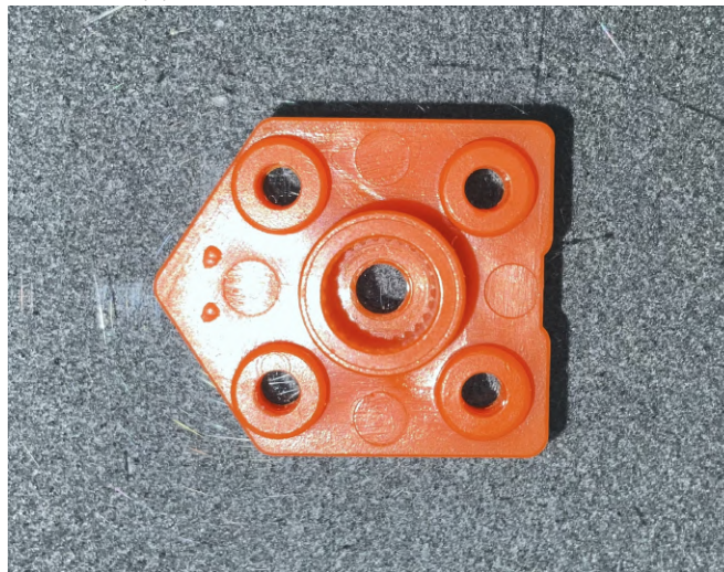
(b) The degraded plastic horn mounted on the given servomotor.
