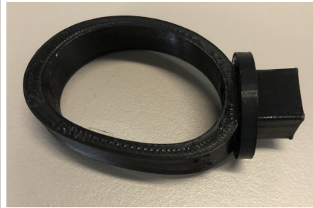
(b) The controller mount for the right Meta Quest or the Meta Quest Pro controller with a male magnet holder superglued to the end.
