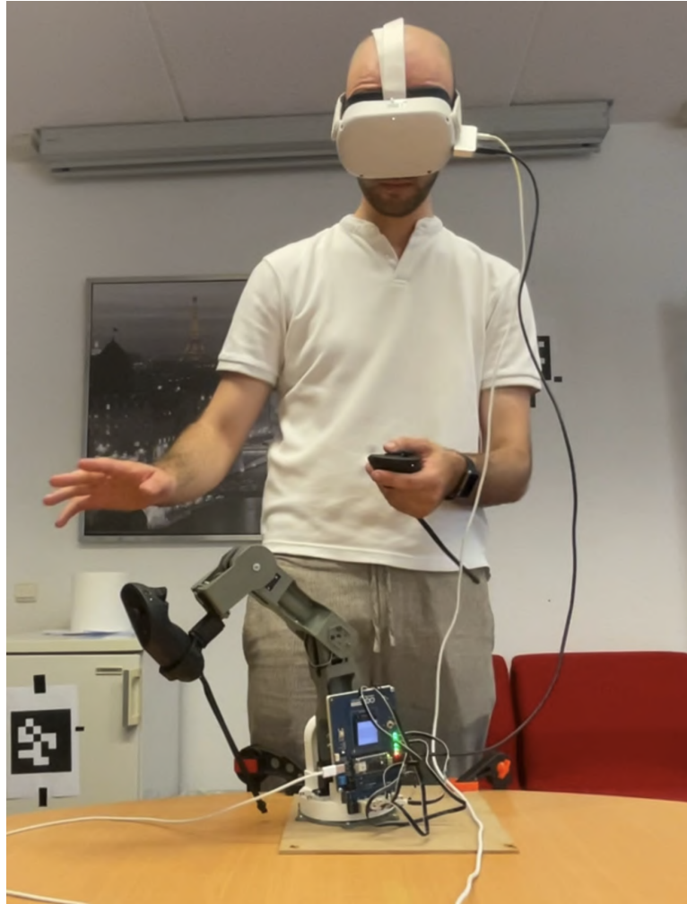
Figure 3.3: ZeroArm in practice using the Meta Quest 2 and the Arduino Braccio++ robot arm seen from an external viewpoint.
