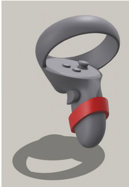
(a) The controller mount, indicated in red, now holding the Meta Quest controller.
