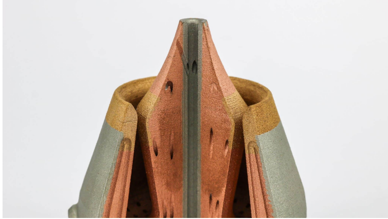
Figure 1.5: Fe-Cu FGM nozzle using Selective Laser Deposition (SLD) [Sher, 2023]
