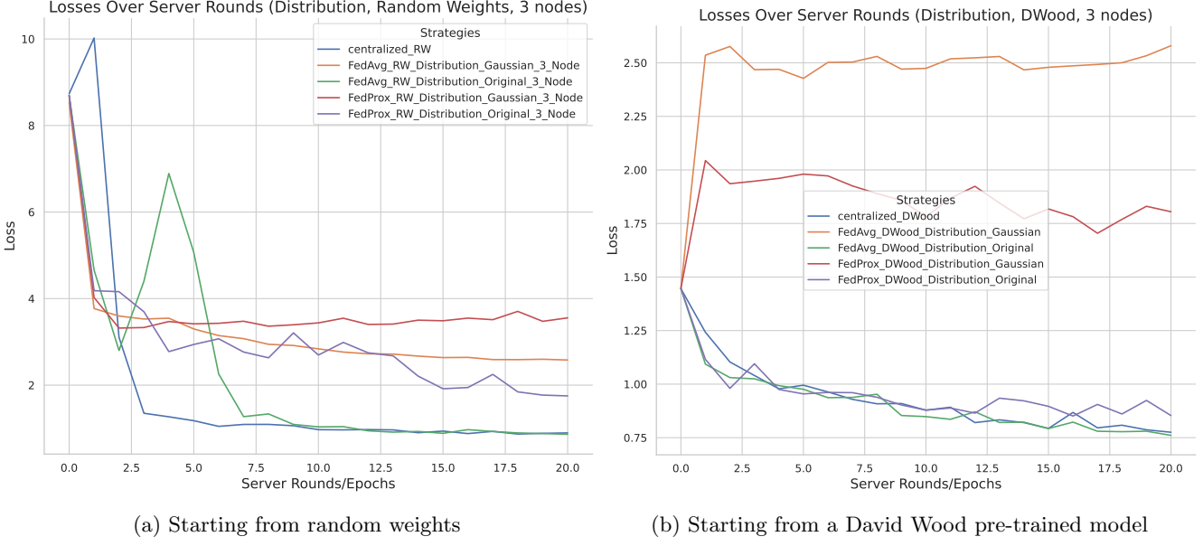
Figure 4.1: Global model losses over server rounds of Federated Learning (across 3 nodes). Calculated using the test dataset.
