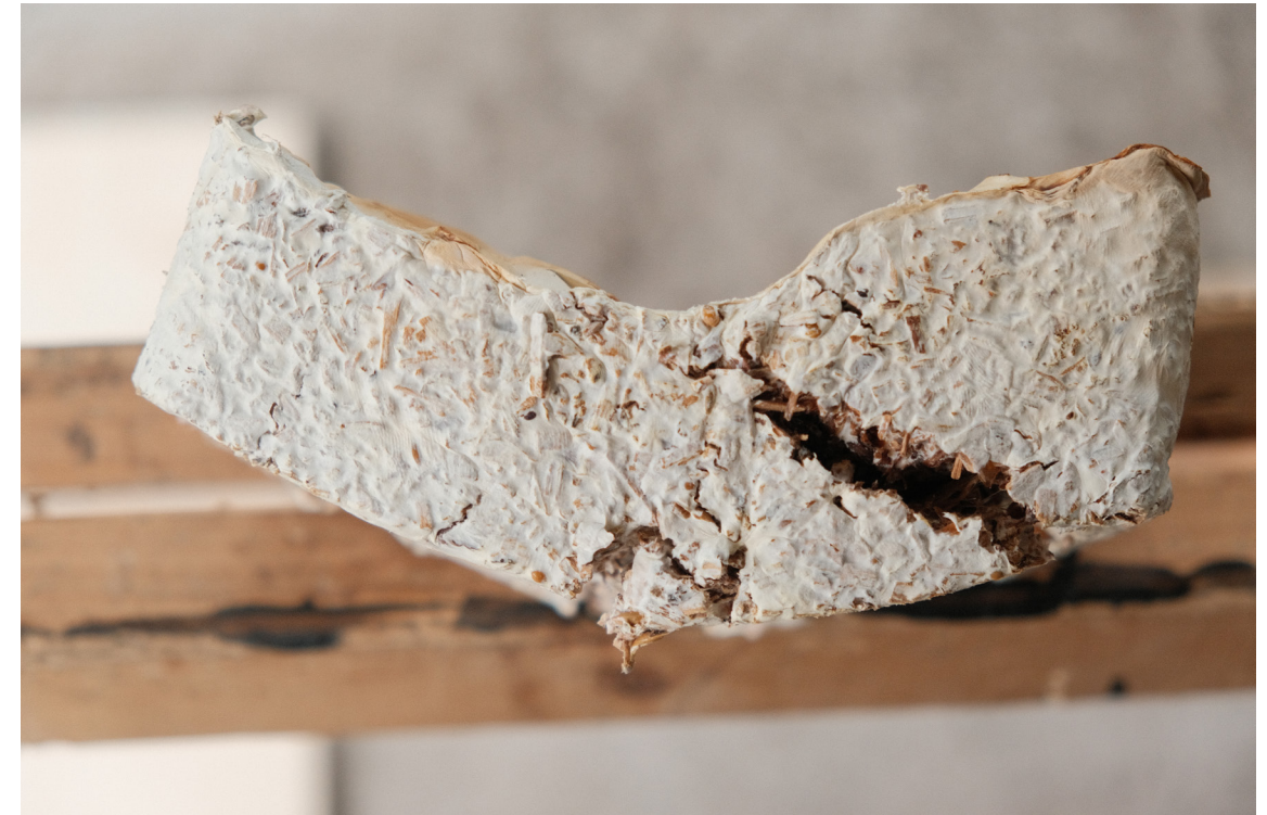
Image: Test piece after executing the three-point bending test
