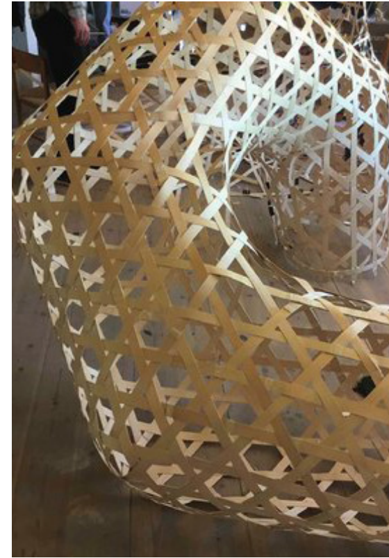
Top: Large scale model made from maple wood strips, all strips are straight making production efficient while still allowing complex shapes (Ayres et al., 2018)
