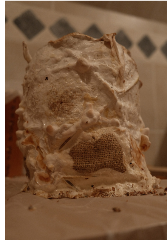
Left: All test pieces removed from PVC cylinders and containers Right top: Proof of concept, uneven growth on the outer layer of jute Right bottom: Placing the plastic sheet over the test pieces to start final growth period of two days
