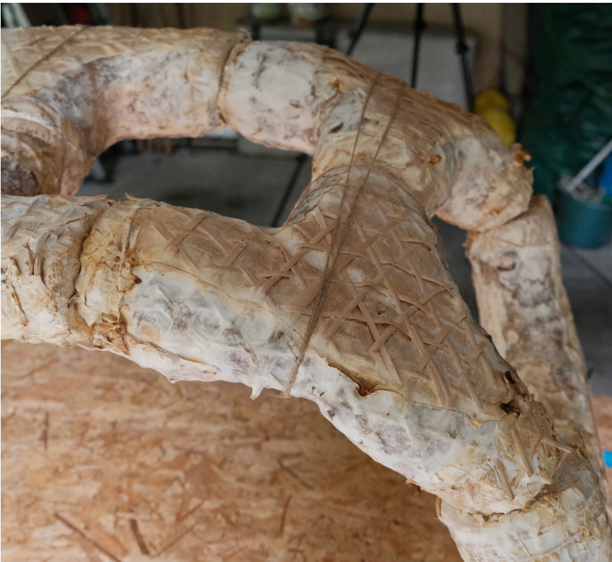
Left: The second arch, made from five correctly grown pieces of the initial arch Top right: Inside view of the top of the arch, all connections fit perfectly Bottom right: Small deformation of the arch due to the shape of the knots, the knots were modelled for a different arch causing this deformation Next page: Detail of a knot
