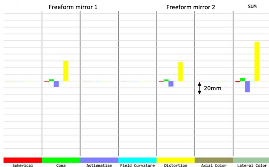
FIGURE 65: SEIDEL DIAGRAM FOR THE FINAL SPECTROMETER'S DESIGN VIS CHANNEL, INDICATING DISTORTION AS THE MAIN ABERRATION
