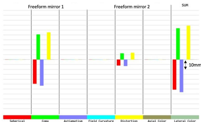
FIGURE 53: SEIDEL DIAGRAM OF THE SINGLE-CHANNEL NIR SPECTROMETER
