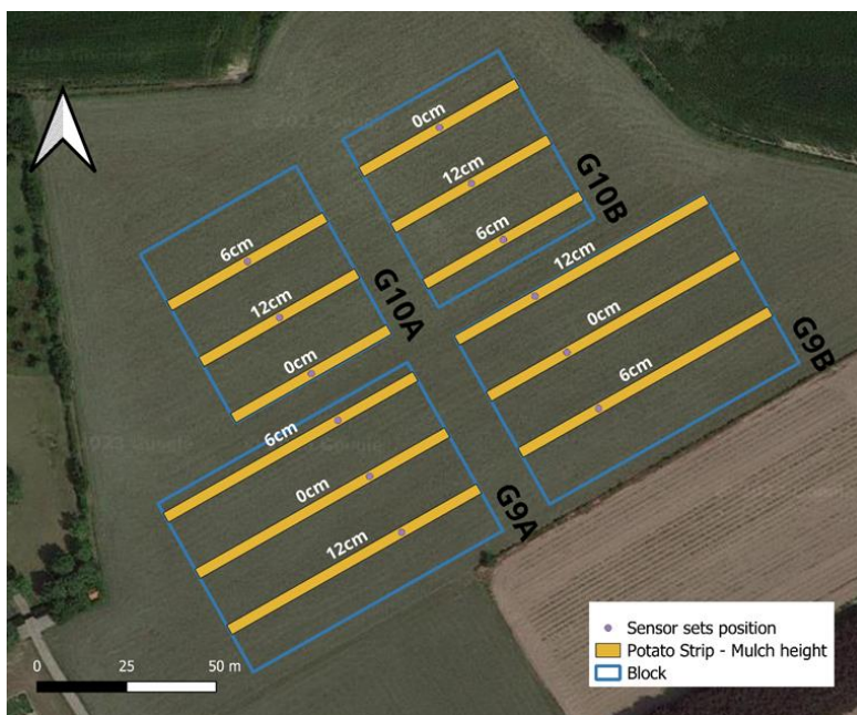
Figure 3: Experimental layout (mulch thickness indicated by 0 cm (no mulch), 6 cm, and 12 cm within each block designated with G9A, G9B, G10A, and G10B)
