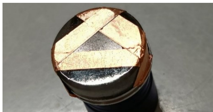
Figure 4-1: Loose powder sintered and prepared for EBSD
