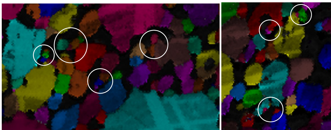
Figure 4-3: Close up of the loose powder EBSD with indicated polycrystals
