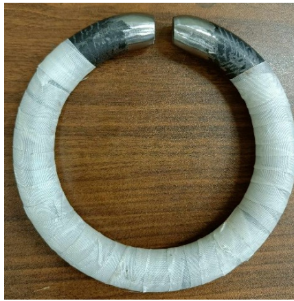
Figure 2-7: Toroidal core with isolation tape applied
