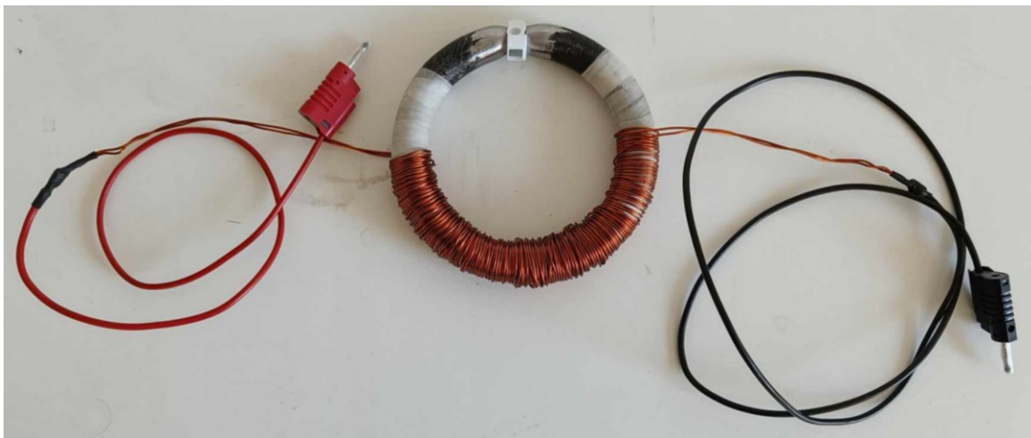
Figure 2-8: Toroidal electromagnet design
