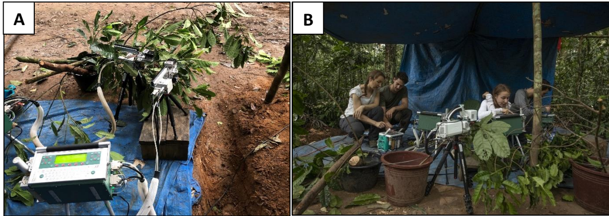
Figure 3.6: Ex-situ measurement on an excised branch, placed in a bucket of water, with the LI-6400XT.
