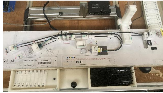
Figure 2: Production of wiring harnesses on harness boards at WAAK.
