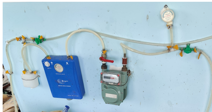
Figure 5.6: Connection between digester outlet and dual-branch test setups
