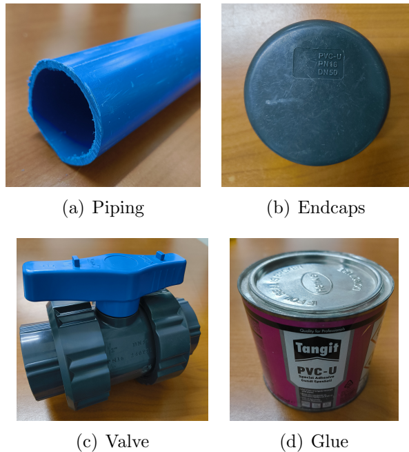
Figure 4.5: Implementation of the water scrubbing setup
