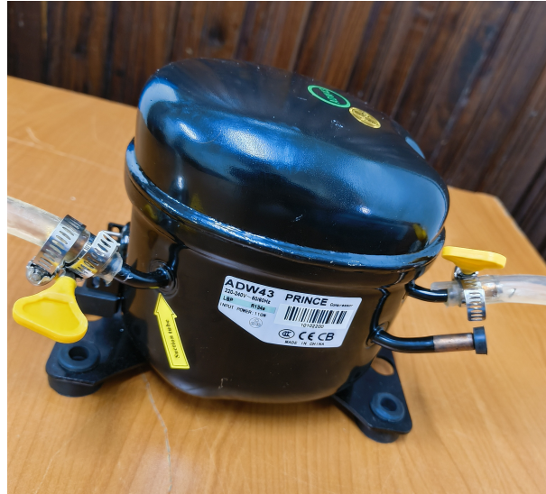
Figure 4.3: Refrigeration compressor ADW43
