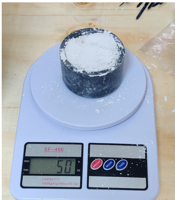
Figure 5.13: Unused endcap holding 50 g of Ca(OH)_2
