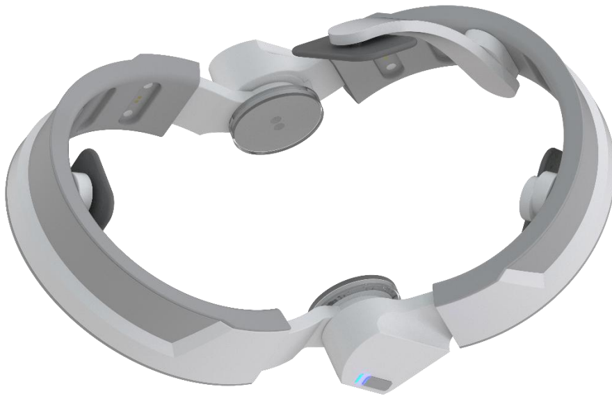
Figure 9-19: Headset with electrodes top view
