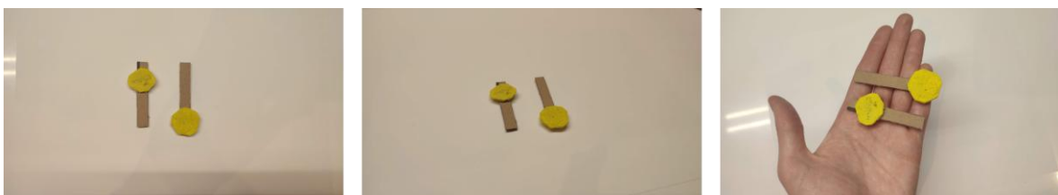
Figure 5-11: First prototype extension arm electrode
