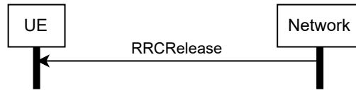
Figure 4.11: The RRC connection release procedure as determined in [3GP24g].
