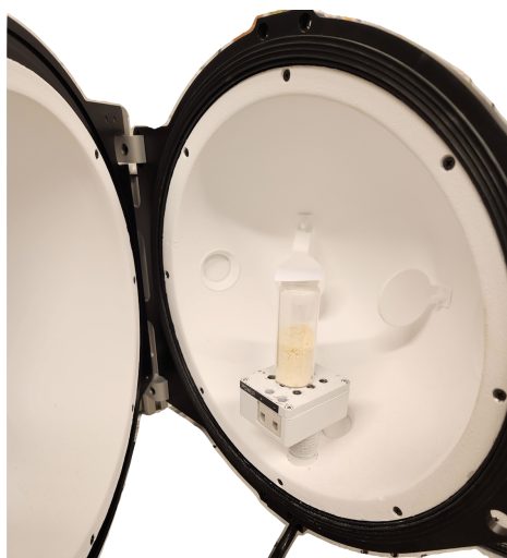
Figure 3.5: Image of the large integration sphere, coated with a Spectralon ® coating.
