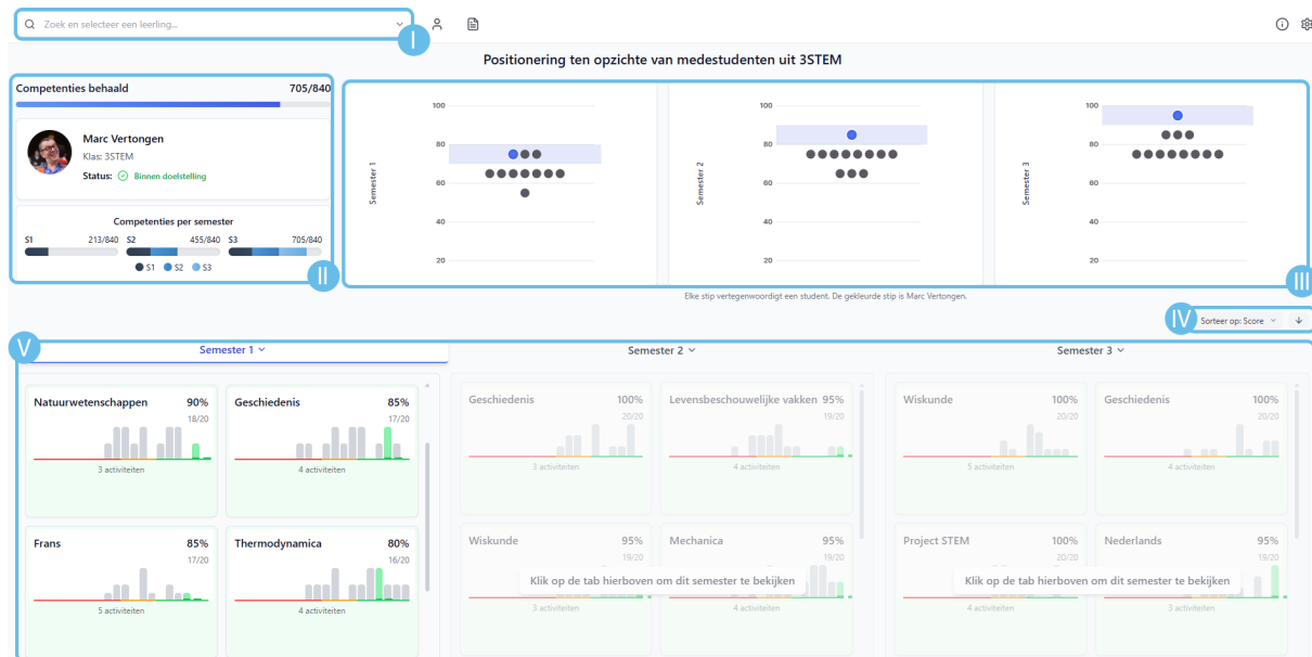
Figure 5.5: Overview of student progress, with five key interface components: I. student filter, II. quick overview of the selected student’s profile, including the number of competencies earned per semester, III. visual representation of the student’s performance evolution relative to the class group, IV. sorting filter for customizing the data display, and V. subject-level performance distributions per semester, showing both individual results and class benchmarks.
