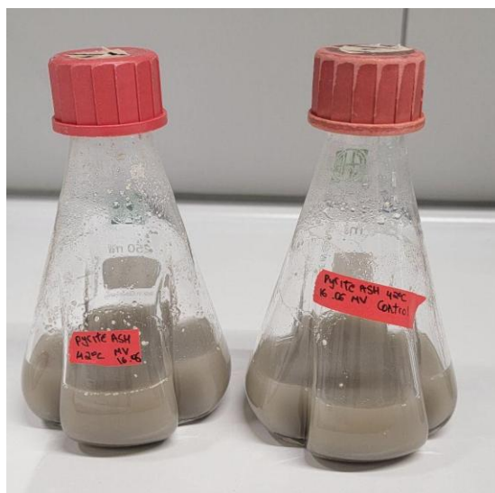
Figure 5.12. Pyrite ashes confirmatory experiments at pH 1.66, 42 °C, pulp density 2% (w/v), Fe (II) 54 mM, and SLA culture and addition of 1% (w/v) sulfur.
